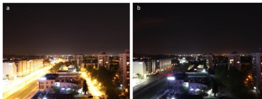
Figure 4. Turning off street lighting in Cracow. Pictures were taken with the same Canon EOS 800D camera settings (ISO 1600, F 5.6, 3 s) about 20 min before midnight (a) and 15 min after midnight (b) on the night of 26–27 April 2020. The only constantly glowing light sources are the petrol station (on the left), some neighbourhood lamps, apartment windows, security lamps, and light advertisements (Photo: Tomasz Ścieżor).
