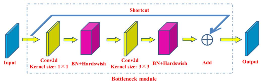
Figure 6. Structure of Bottleneck module.
