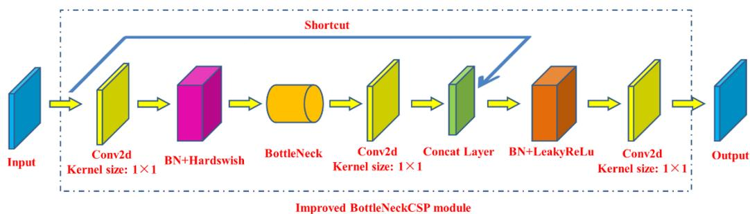
**Figure 9.** Structure of improved BottleneckCSP module (BottleneckCSP-2 module).
