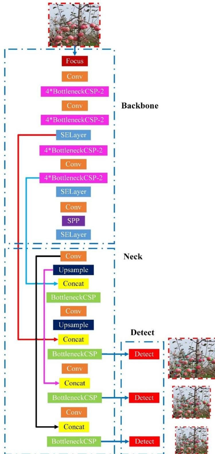
Figure 10. Architecture of improved YOLOv5s network.
