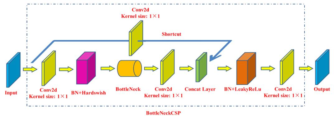
Figure 7. Structure of BottleneckCSP module.
