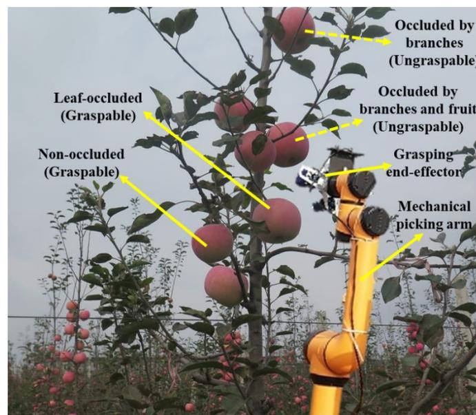
**Figure 1.** Schematic diagram of practical harvesting situation that picking robot confronts.
