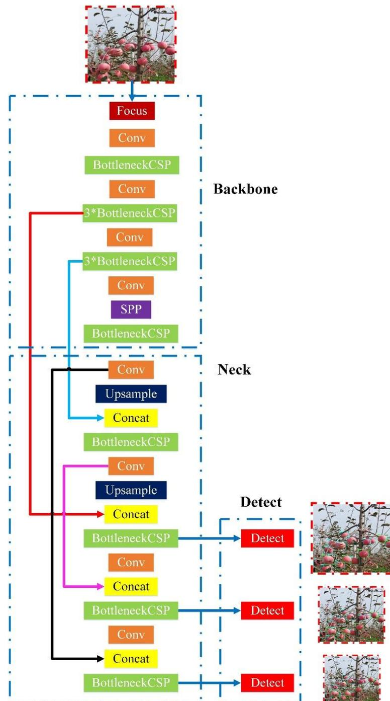
**Figure 4.** Architecture of original YOLOv5s network.
