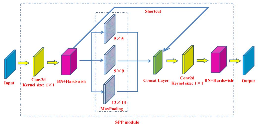
Figure 8. Structure of SPP module.
