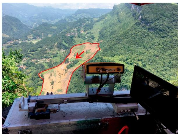
**Figure 3.** GB-InSAR system employed in the emergency monitoring.
