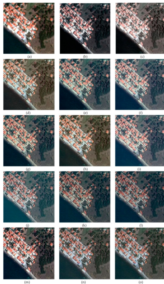
Figure 6. Zoom of the RGB composition of the initial multispectral images (a) and zoom of the RGB composition of the multispectral pan-sharpened images obtained from each method, respectively: (b) MLT; (c) SM; (d) GS; (e) BT; (f) IHS; (g) BTF; (h) GSF; (i) IHSF; (j) HPF; (k) SFIM; (l) MTF-GLP-HPM; (m) MTF-GLP; (n) GS2; (o) MTF-GLP-CBD.
