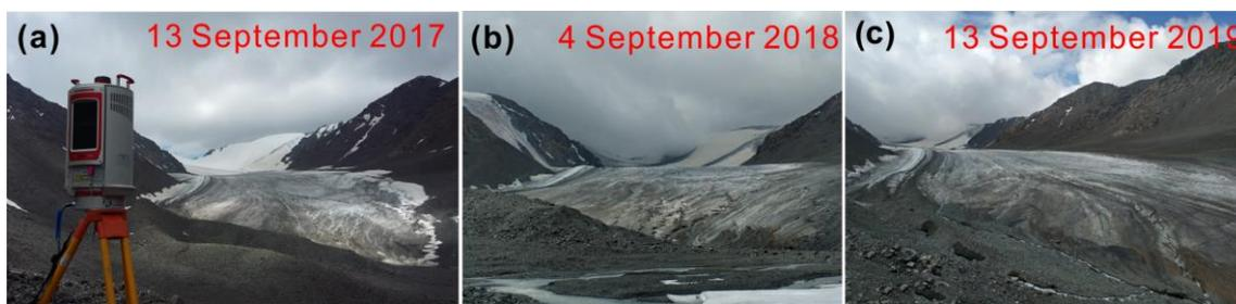
**Figure 3.** TLS survey of the Muz Taw Glacier with the Riegl VZ<sup>®</sup>-6000 TLS in September 2017 (a), 2018 (b), and 2019 (c). The ablation area was mainly covered with bare ice.
