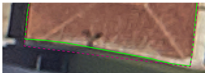
Figure 13. Incorrect boundary extraction caused by the white feature on the edge, extracted boundary (green), and correct boundary (dashed magenta).
