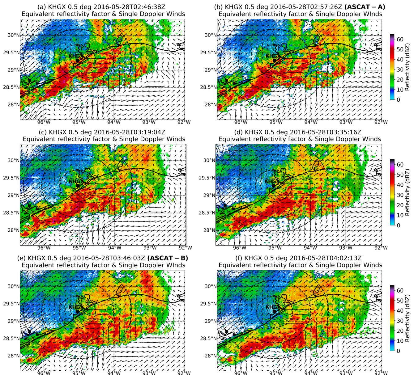
**Figure 1.** Time series depiction of reflectivity field and single-Doppler winds for KHGX radar station. Concentric circles (black dashed) are drawn at 50 km intervals, i.e., at a distance of 50, 100 and 150 km from the radar location. (b,e) correspond to the closest times of the ASCAT-A and -B overpass, respectively.
