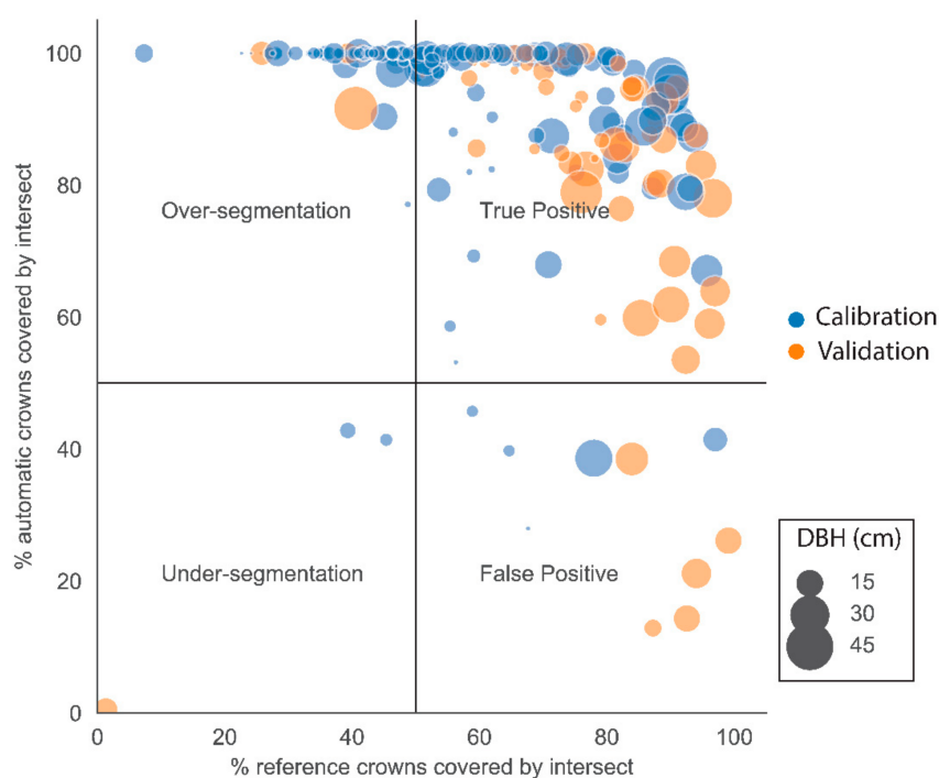
Figure 5. Scatter plot showing the percentage of intersection between manually and automatically delineated crowns. Point sizes are proportional to field measured DBH. Note that when more than one automatically segmented crown overlapped with a manually delineated crown, the automatic crown with the largest percentage cover was used in the analysis.
