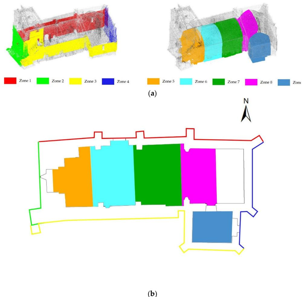
**Figure 8.** Test zones considered for evaluating the performance of the noise reduction filter: (a) 3D view and (b) plant view.
