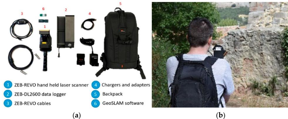
**Figure 5.** Wearable mobile mapping system used: (a) main components and (b) photo taken during the data acquisition.
