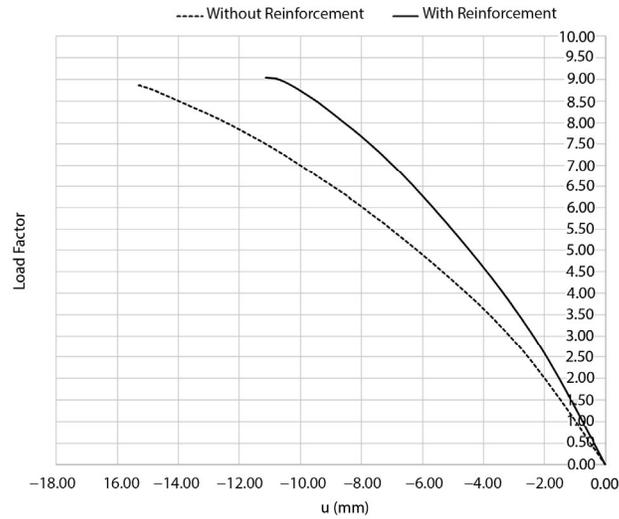
**Figure 17.** Load–displacement curves obtained during the static non-linear analysis. The dash line represents the structure with the TRM layers.
