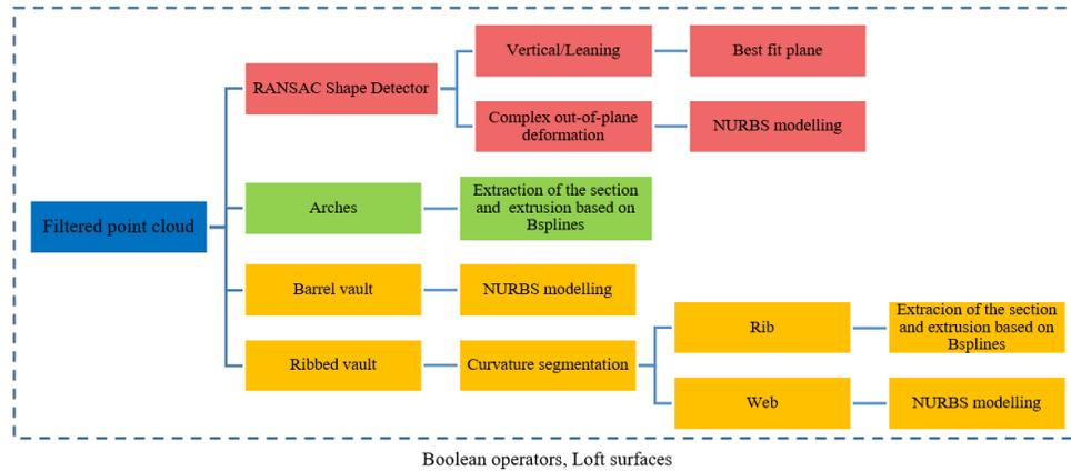
**Figure 12.** Graphical workflow proposed for creating the as-built CAD model. The red rectangles are those stages used for modelling the masonry wall. The green and orange rectangles include the strategies for modelling the arches and the vaults, respectively. RANSAC: random sample consensus.
