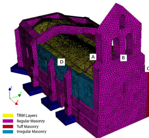
**Figure 16.** General view of the numerical mesh. The point A refers to the control node placed at the intrados of the barrel vault. Point B refers to the control node used for the pushover analysis in the +X direction. The control node placed at the same height but at the intrados of the tower was used for the analysis in the -X direction. Points C, D refer to the nodes used for the pushover analysis in the direction +Y and -Y, respectively.
