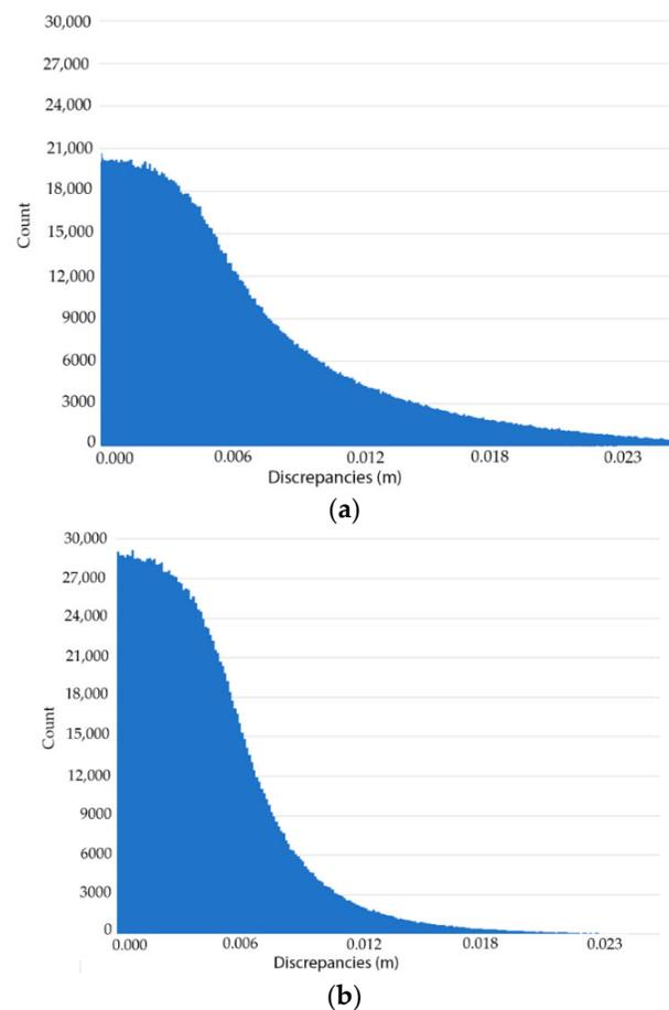
**Figure 9.** Histograms of the relative discrepancies between the terrestrial laser scanner (TLS) and the WMMS in the test zone 3: (a) before applying the filter, the maximum error is 3 cm and around 80% of the data are below 1 cm of error and (b) after the application of the noise reduction filter, the maximum error is 2 cm and 95% of the data are below 1 cm of difference.
