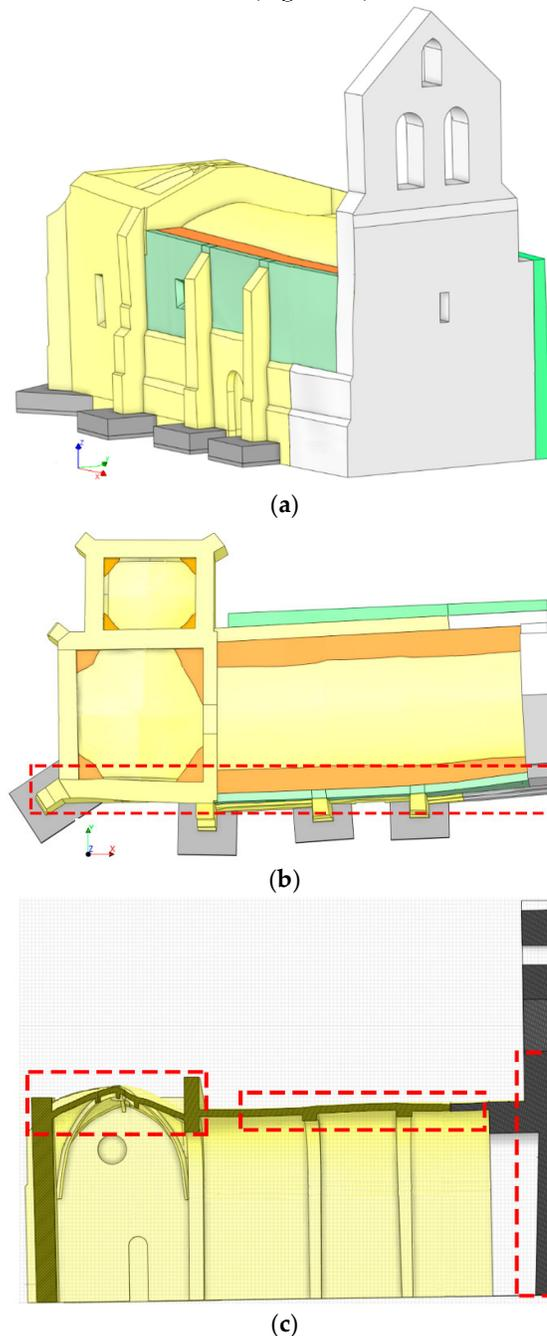
**Figure 15.** As-built CAD model: (a) general view; (b) plant view and (c) transversal section. In red it is highlighted some areas of the church with complex deformations properly modelled by the proposed approach. In yellow, grey and green the different masonries identified, in orange the infill of the vaults.
