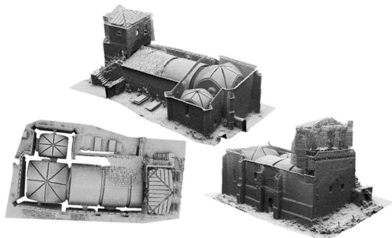
Figure 7. General view of the point cloud obtained.
