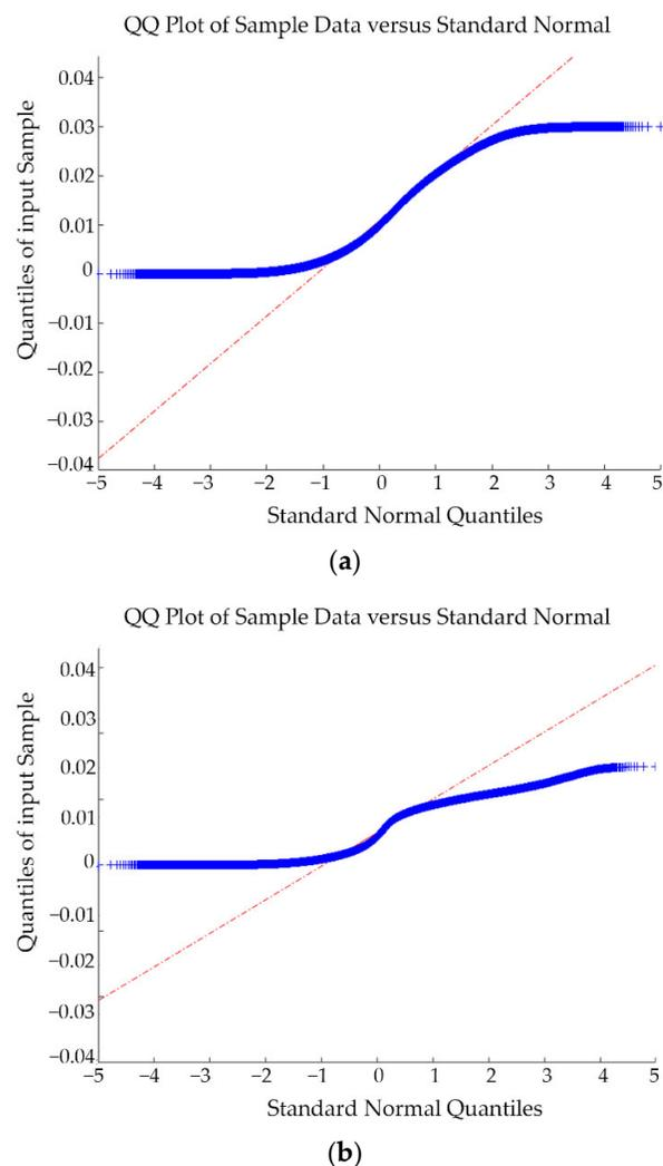
**Figure 10.** QQ-plots of the relative discrepancies between the TLS and the WMMS in the test zone 3: (a) before and (b) after the application of the noise reduction filter. In blue, the deviation of the quantiles position of the sample in comparison with expected quantiles for a normal distribution. In red, the trend line for a perfect Gaussian population.
