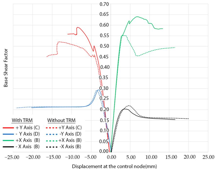
**Figure 20.** Mass-proportional pushover capacity curves in the four main directions (red colour for the  $+Y$ , green colour for  $+X$ , blue for the  $-Y$  and black for the  $-X$ ). Dash lines represent the behaviour of the structure without the TRM layer. The control points used for each curve has been placed between markers.
