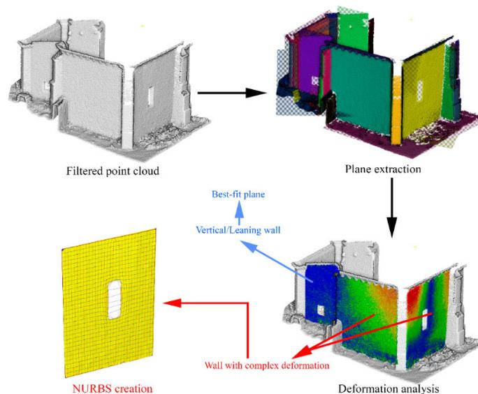
**Figure 13.** Workflow used for modelling walls.
