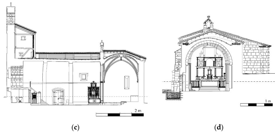
**Figure 2.** Planimetry of the church: (a) main elevation; (b) top view; (c) longitudinal section and (d) transversal section.
