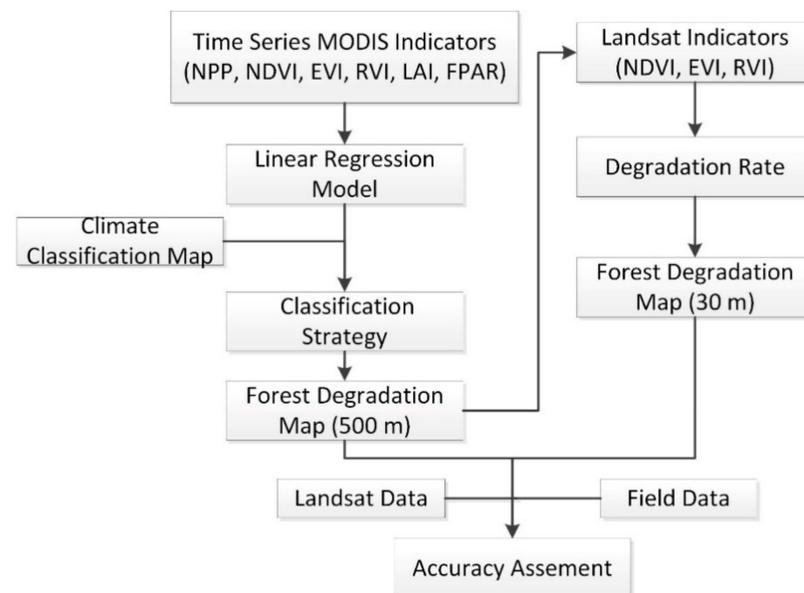
**Figure 2.** Flowchart of detecting forest degradation from MODERate Resolution Imaging Spectroradiometer (MODIS) and Landsat Enhanced Thematic Mapper Plus (ETM+) data. Regression models were adopted to analyze the trend from MODIS Products, then a classification model was established to analyze the degradation level, ETM+ data were used to obtain details in the degraded MODIS pixels.
