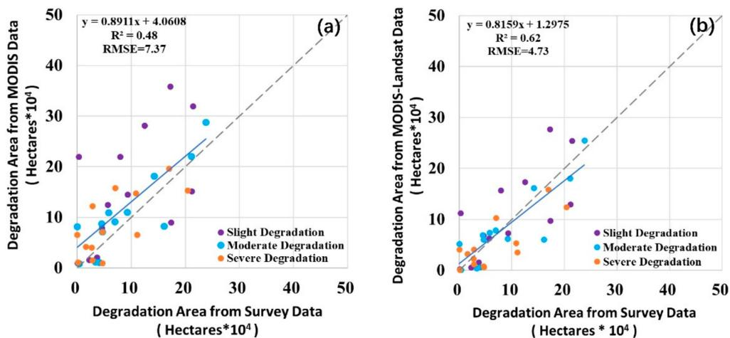
**Figure 7.** Validation of degradation area from remote sensing data against ground survey data. (a) is the validation from MODIS data, and (b) is the validation from MODIS-Landsat data. Forest degradation from MODIS-Landsat data achieved a better precision.
