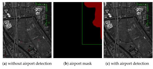
**Figure 10.** Effectiveness of the proposed airport detection algorithm. The green box represents the correctly detected aircraft, and the red box represents false alarms.
