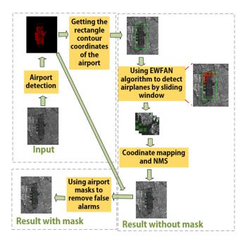
Figure 1. The efficient framework for aircraft detection.
