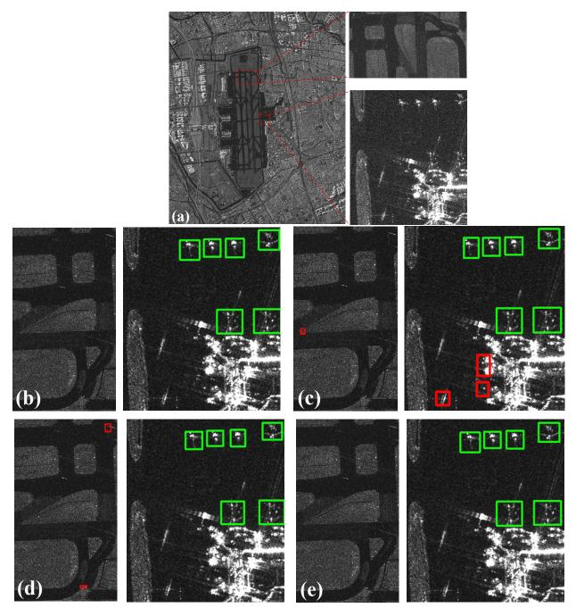
**Figure 11.** The experiment result for Airport I. (a) SAR image of Airport Ifrom Gaofen-3. (b) The ground truth of the airport. (c-e) the aircraft detection results of (a) by EfficientDet, YOLOv4, and EWFAN. The green box, the red box, and the yellow box represent the correctly detected aircrafts, the false alarms, and the missed alarms respectively.
