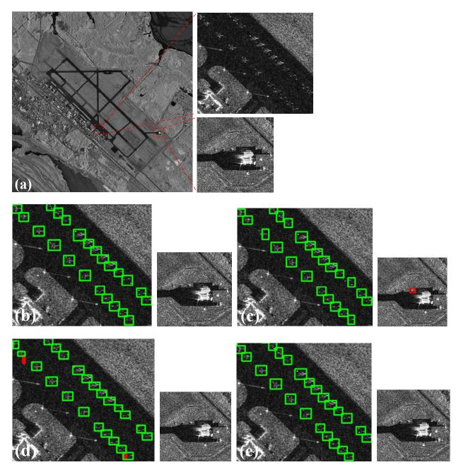
Figure 12. The experiment result for Airport I. (a) SAR image of Airport I from Gaofen-3. (b) The ground truth of the airport. (c-e) the aircraft detection results of (a) by EfficientDet, YOLOv4, and EWFAN. The green box, the red box and the yellow box represent the correctly detected aircrafts, the false alarms, and the missed alarms respectively.
