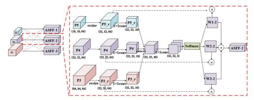
Figure 5. Schematic diagram of Adaptively Spatial Feature Fusion (Taking ASFF-2 as an example).
