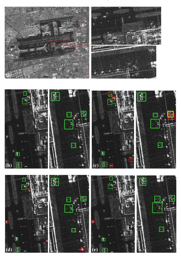
**Figure 13.** The experiment result for Airport I. (a) SAR image of Airport I from Gaofen-3. (b) The ground truth of the airport. (c-e) the aircraft detection results of (a) by EfficientDet, YOLOv4, and EWFAN. The green box, the red box, and the yellow box represent the correctly detected aircrafts, the false alarms, and the missed alarms respectively.
