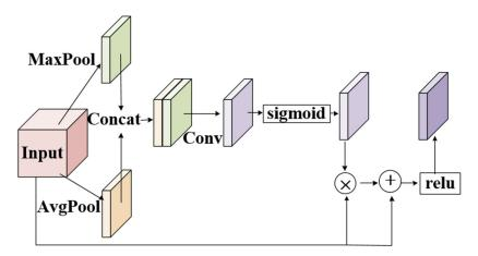
Figure 4. Schematic diagram of Residual Spatial Attention Module.
