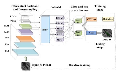
**Figure 2.** The framework of the Efficient Weighted Feature Fusion and Attention Network (EW-FAN) algorithm.
