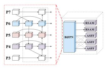
Figure 3. The structure of weighted bi-directional feature pyramid network.
