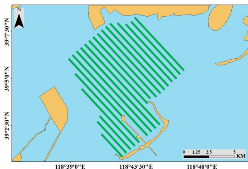
Figure 2. The ship route, with a spacing of ~500 m, for the acoustic survey of the seagrass distribution.
