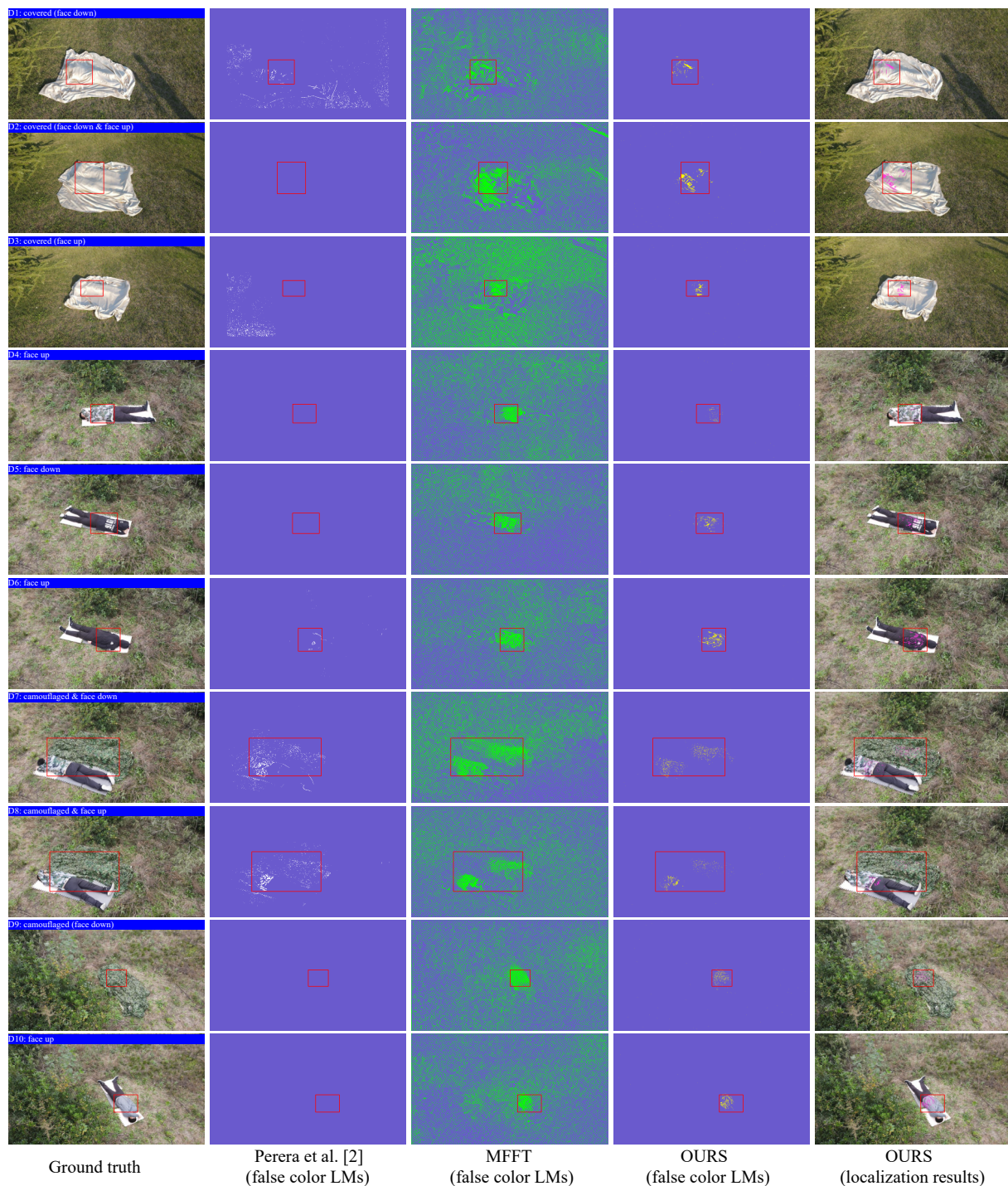
Figure 6. False color location maps (LMs) of Perera et al.' work [2], MFFT and ours, and our localization results for ten drone videos.
