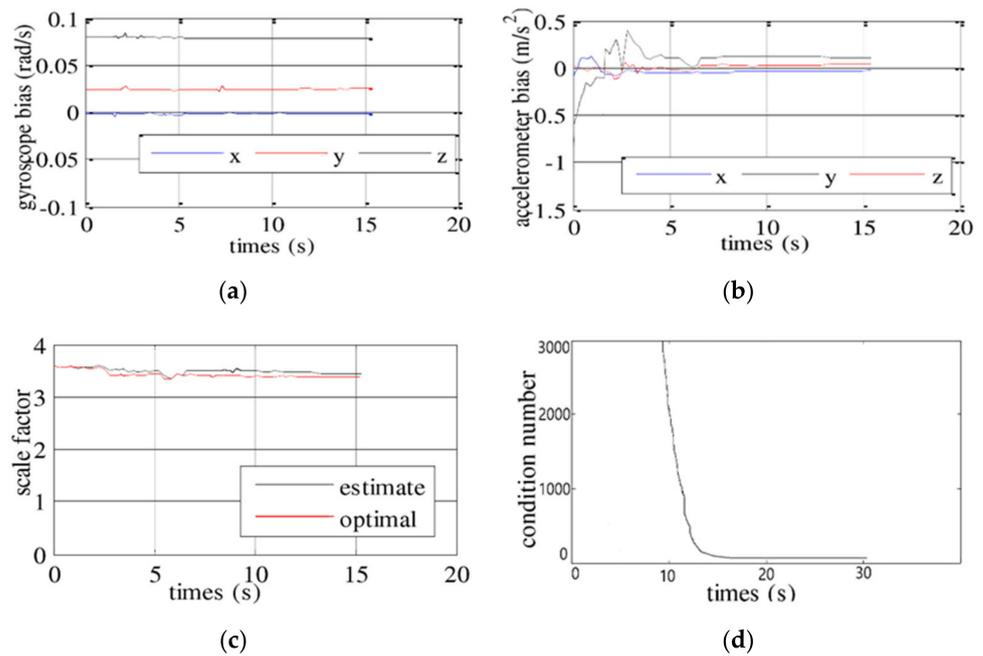
**Figure 6.** This figure describes the results of initialization of variables in dataset MH\_01\_easy dataset. (a,b) describe separately the result of gyroscope bias initialization and accelerometer bias. (c) describes the results of initialization of scale. (d) describes the convergence of the number of system variables.
