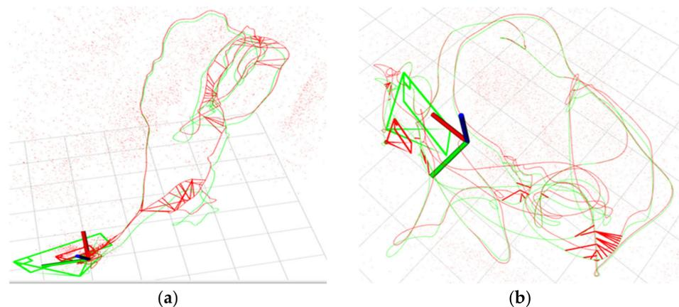
**Figure 10.** Improved VINS-mono Running results of the system in dataset MH\_01\_easy (a) and dataset V2\_02\_medium (b) (red line represents real trajectory, green line represents estimate trajectory).
