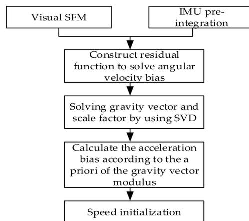
**Figure 2.** Procedure of initializing of the improved VINS-mono.
