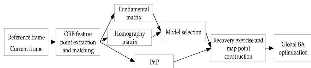
**Figure 3.** Visual Structure from Motion (SFM) flowchart.
