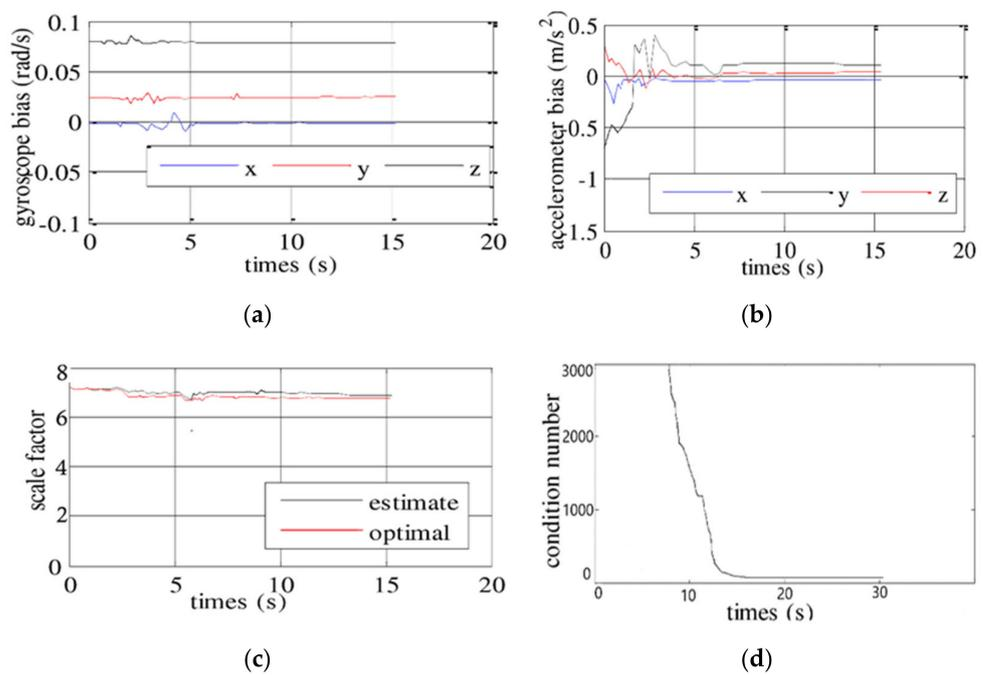
**Figure 7.** This figure describes the results of initialization of variables in dataset V1\_02\_media dataset. (a,b) describe separately the result of gyroscope bias initialization and accelerometer bias. (c) describes the results of initialization of scale. (d) describes the convergence of the number of system variables.
