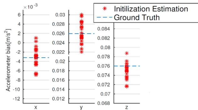
**Figure 8.** Accelerometer bias in the initialization procedure in MH\_01\_easy dataset. The figure contains the results in 20 tests with different start time.
