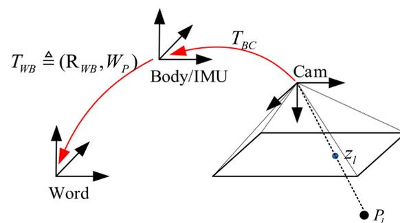
Figure 4. Conversion relations of different coordinate systems.
