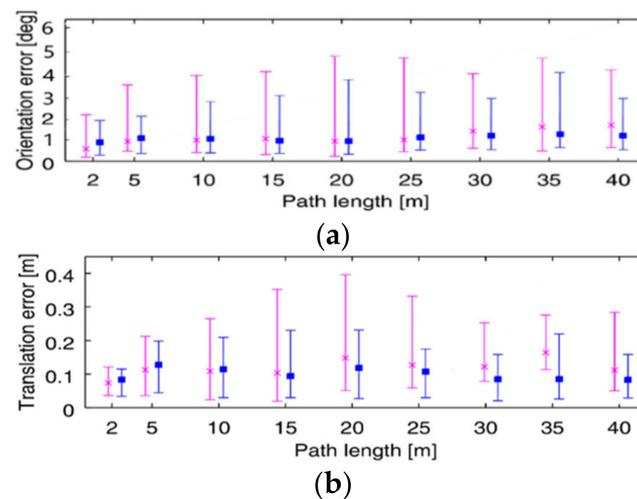
**Figure 12.** This figure describes error comparison analysis in dataset MH\_01\_easy. (a) Orientation error and (b) Translation error (red for VINS-mono system and blue for the improved VINS-mono system).
