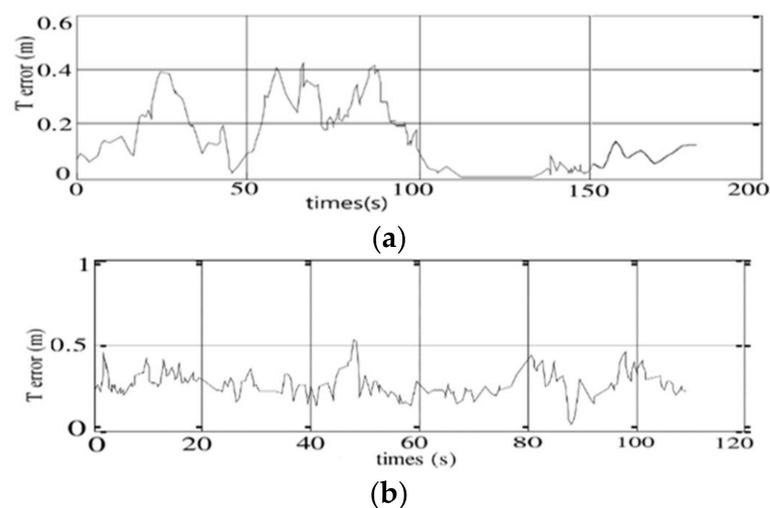
**Figure 11.** The graph describes the trajectory error change of the improved system over time in dataset MH\_01\_easy (a) and Dataset V2\_02\_medium (b) testing.
