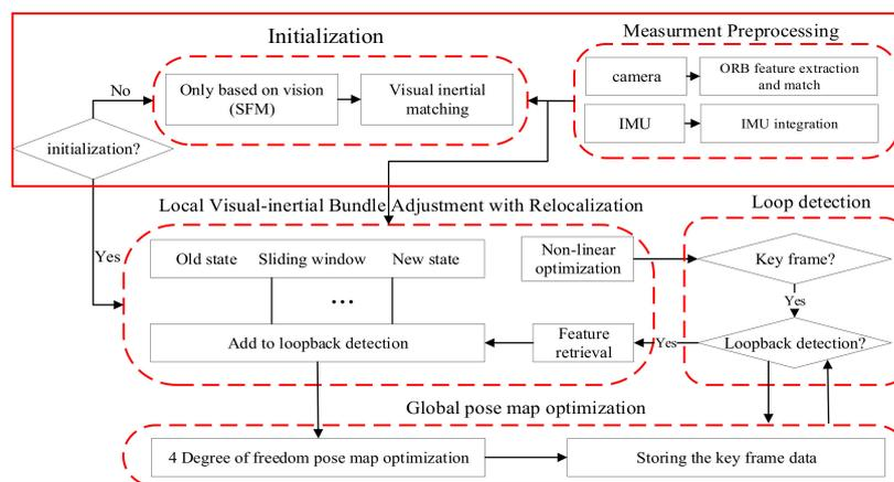
**Figure 1.** The improved visual-inertial navigation system (VINS)-mono system architecture framework.
