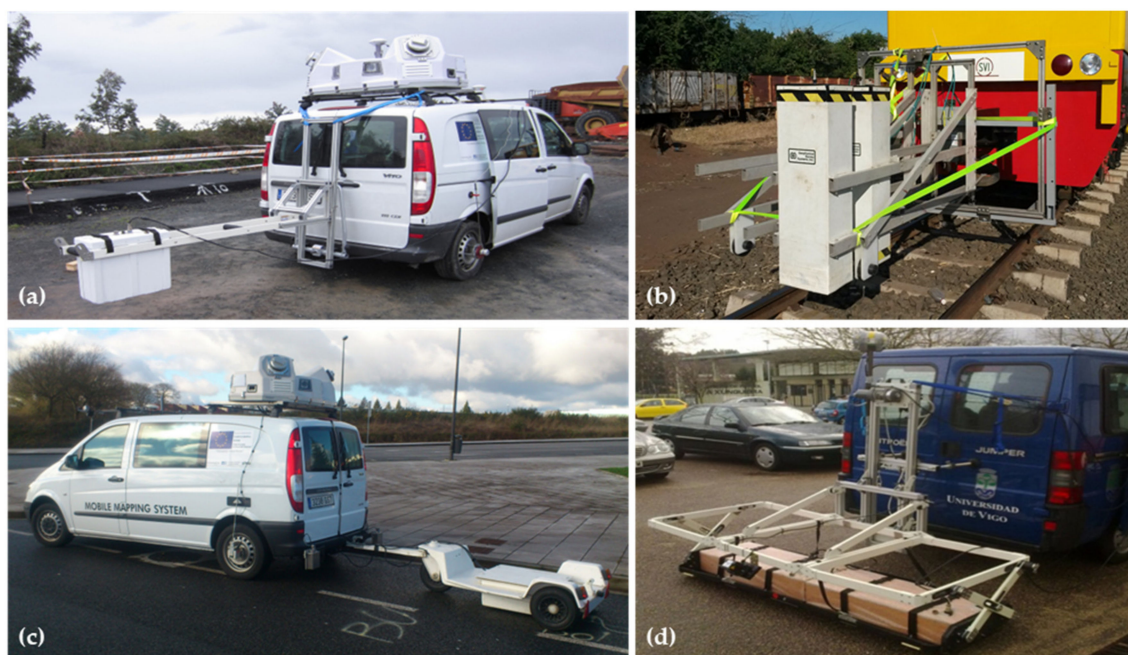
Figure 1. Different ground penetrating radar (GPR) antennas: (a) air-coupled (horn) antennas, (b) multi-antenna system (horn), (c) ground-coupled (dipole) antennas in a trolley, and (d) array multi-channel (ground-coupled) antennas.
