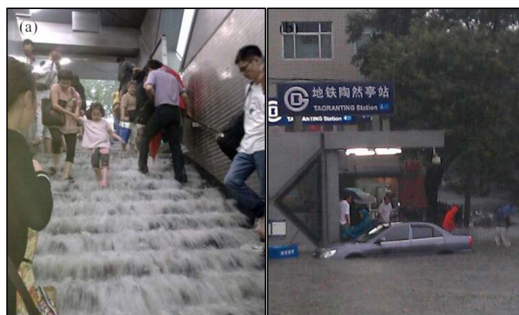
Figure 1. The Beijing subway station was flooded during heavy rainfall on 23 June 2011. (a) Flood-water entered into the southwest exit (Exit D) of the Taoranting station along the escalator. (b) Road waterlogging outside the Taoranting subway station (Exit D).
