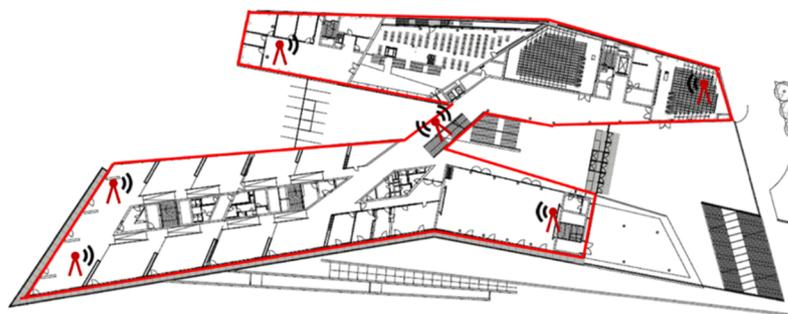
**Figure 5.** Concept drawing for an additional indoor antenna to evaluate the need of indoor units in different indoor environments.
