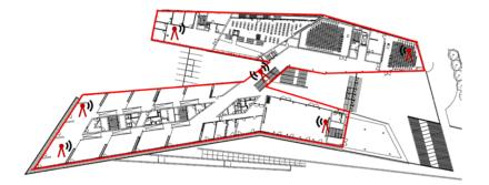
**Figure 5.** Concept drawing for an additional indoor antenna to evaluate the need of indoor units in different indoor environments.
