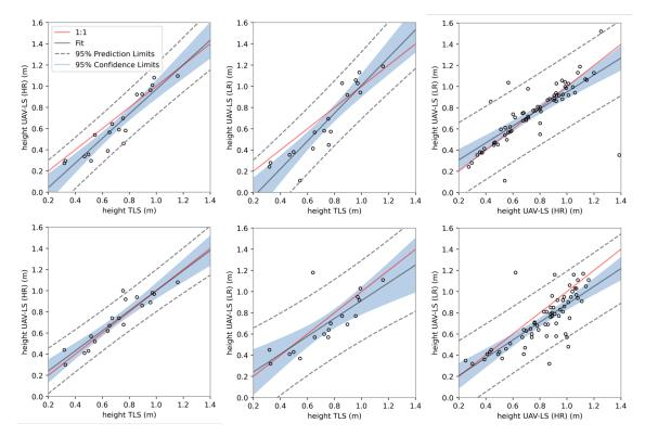
**Figure 11.** Scatter plot with linear regressions of the height estimations, validated using the benchmark data set. The top three plots show results from the Gaussian approach and the bottom three from the grid approach.
