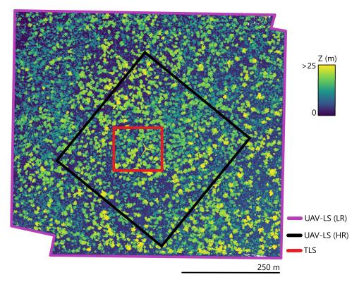
**Figure 1.** UAV-LS (low resolution) point cloud, indicating the boundaries of all data types. The colour code represents the height above terrain. The maximum tree height is approximatively 25 m, and the open canopy allows a substantial understorey.
