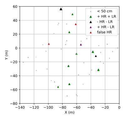
**Figure 8.** Locations of the mounds derived from the 1 ha benchmark data set. + (plus) means the mound is detected; - (minus) means it is not detected by the UAV-LS detection algorithm. The grey mounds are small mounds <50 cm that could only be detected in the benchmark data set.
