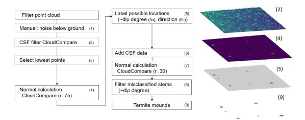
Figure 3. Overview of the main steps to extract termite mounds from UAV-LS data. CSF, cloth simulation filter.
