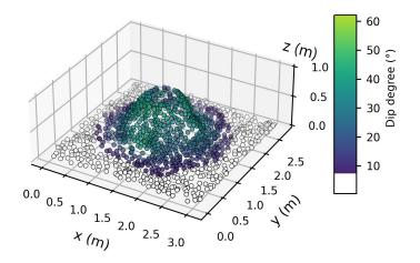
**Figure 4.** A termite mound in the UAV-LS (HR) point cloud. Points are first filtered based on dip degree; if this value falls outside the interval [7°, 86°], points are rejected. Then, data are clustered, and only point clusters that have more than 50 points are considered. The white points are the rejected points.
