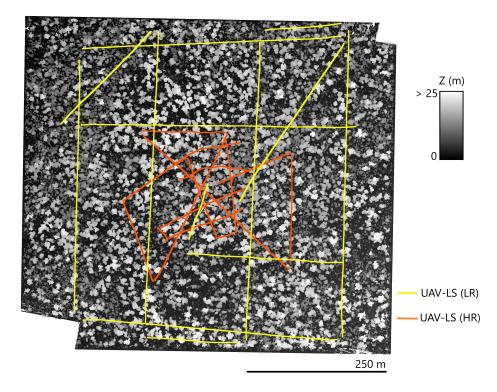
**Figure A1.** UAV-LS (LR) point cloud. The colour code represents the height above the terrain. The lines represent the recorded flight lines of F1 (UAV-LS (HR)) and F2 (UAV-LS (LR)). Only sections of the flight lines that were used in the registered point clouds are visualized.
