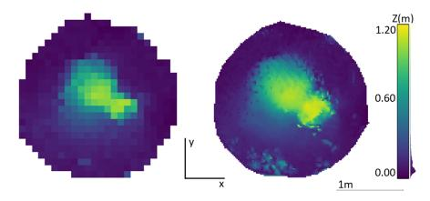
**Figure 6.** To estimate termite mound height, a large grid size was used to avoid the influence from outliers (**left**). To calculate volume, a smaller grid size was used. Since the volume was calculated as the sum of many small cuboids, possible outliers had less influence (**right**).
