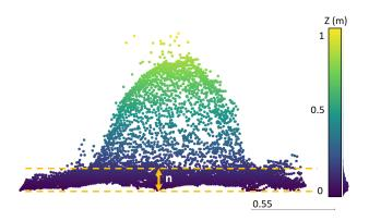
**Figure 7.** Rasterized point cloud for volume calculation (UAV-LS (HR)). The cuboids that are used to estimate the volume are confined by the top line and the termite mound. The bottom line represents the average height of the lowest 20 points. The value of n was optimized to prevent over- or under-estimations of termite mound volume.
