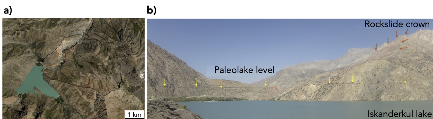
Figure 2. Iskander lake. (a) Google Earth view of the Iskander lake dammed by a rockslide. Black polygons correspond to the landslide catalogue. (b) Field view of the Iskander lake dam. Rockslide crown highlighted by red arrows; paleolake level, marked by yellow arrows, represent the maximum lake level before the dam incision commenced.
