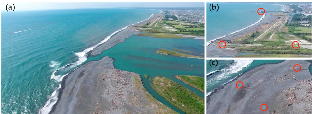
**Figure 3.** An example frame of the video and ground control points (GCPs) indicated by red circles (Case 4): (a) a video frame by UAV and (b,c) enlarged views of ground control points.
