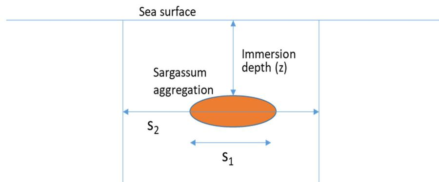
**Figure 6.** Schematic configuration of the way the influence of *Sargassum* aggregation located at a given depth is represented in Lee's radiative transfer model [19]. The *Sargassum* aggregation is located at an immersion depth  $z$ .  $S_1$  is the area covered by the *Sargassum* aggregation and  $S_2$  is the total area of a given pixel.
