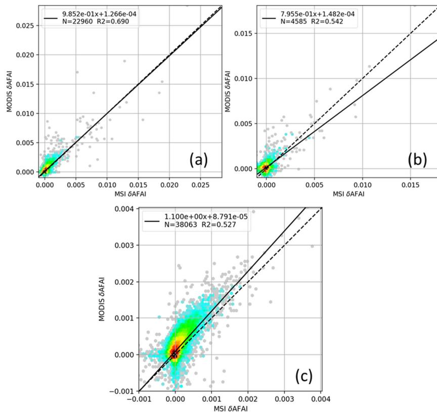
**Figure 7.** Comparison between MODIS/ $\delta$ AFAI and MSI/ $\delta$ AFAI for the three study areas: (a) site #1, (b) site #2 and (c) site #3. The statistical parameters, namely the coefficient of determination  $R^2$ , the slope and y-intercept are reported within each figure. The 1:1 and regression lines are shown using dashed and continuous lines, respectively.
