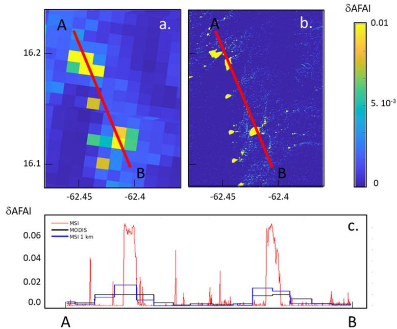
**Figure 3.** (a) MODIS/ $\delta$ AFAI/(a) and (b) MSI/ $\delta$ AFAI on 21 June 2018 for the same site (site #1), and (c)  $\delta$ AFAI values along the AB transect where the red line corresponds to MSI-20 m, the black line to MODIS 1 km, and the blue line to MSI-1 km.
