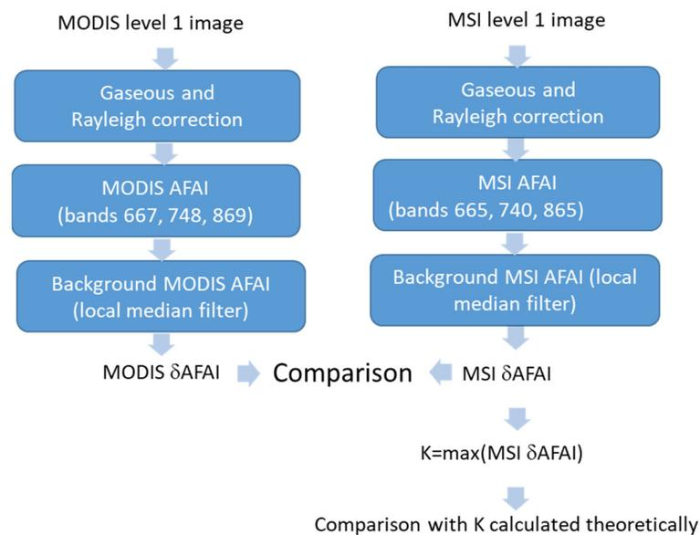
**Figure 5.** Flowchart of the overall methodology used to compare MODIS/ $\delta$ AFAI and MSI/ $\delta$ AFAI and to empirically estimate the slope  $K$  of the linear relationship between  $\delta$ AFAI and the fractional coverage (FC).
