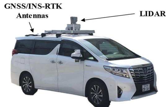
**Figure 7.** Experimental platform with sensor configurations.
