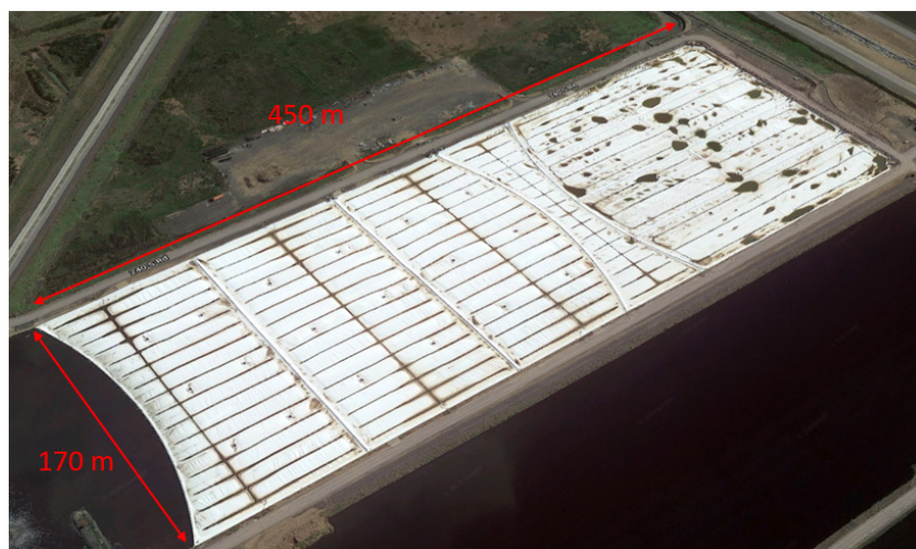
Figure 1. Google Map view of one of the HDPE geomembrane floating covers on an anaerobic lagoon at the WTP in Werribee, Victoria, Australia.
