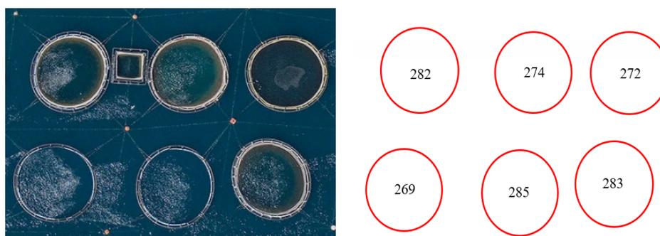
**Figure 10.** A fish farm satellite image (Left) and the extracted circles from the image and radii results (Right) using VFCSS algorithm.
