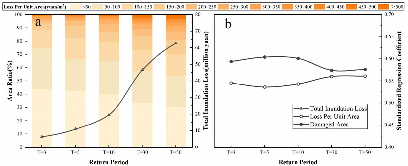
Figure 11. (a) Distribution of the ratios of the damaged areas to the total damaged areas in the groups, and the total inundation loss under different return periods; (b) standardized regression coefficients under different return periods.
