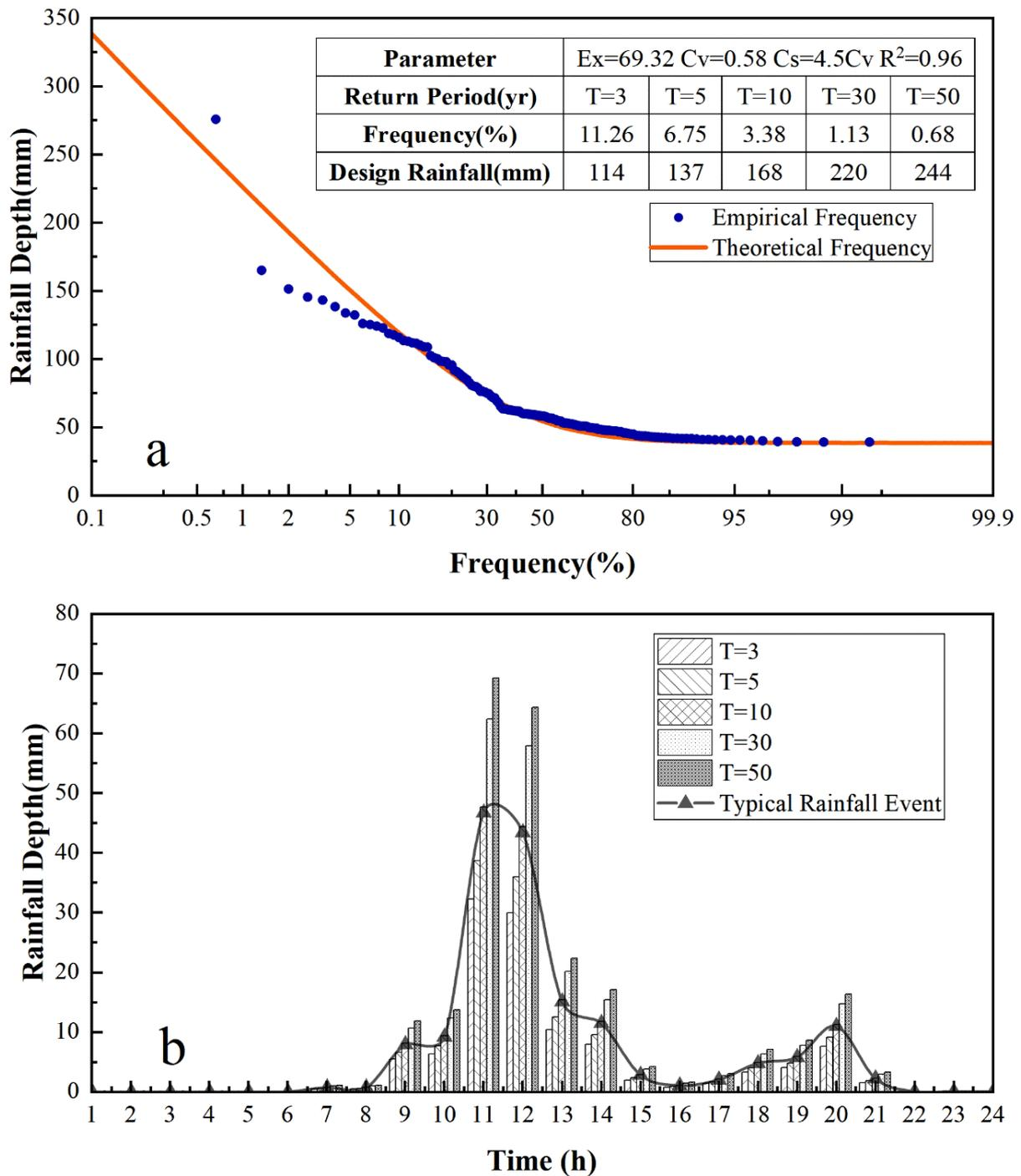
**Figure 2.** (a) The frequency curve of the designed rainfall; (b) typical rainfall process and designed rainfall process under different return periods.
