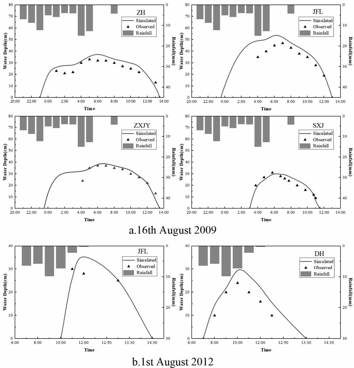
**Figure 5.** Observed and simulated water depths of the two historical rainfall events: (a) 16 August 2009; (b) 1 August 2012.
