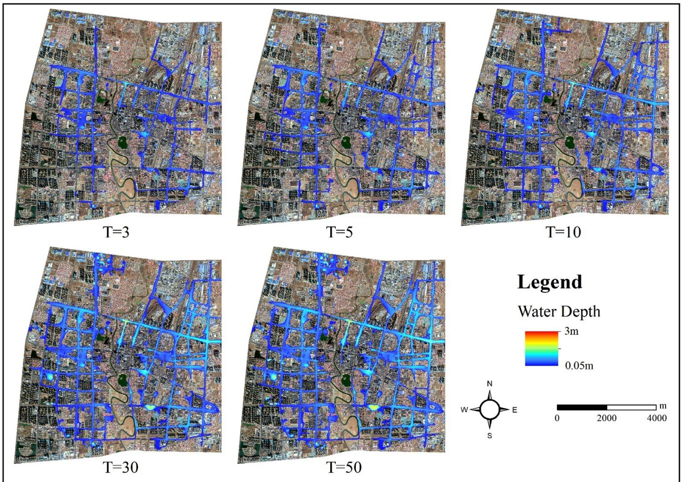
Figure 6. Spatial distribution of the maximum inundation depth under different return periods.
