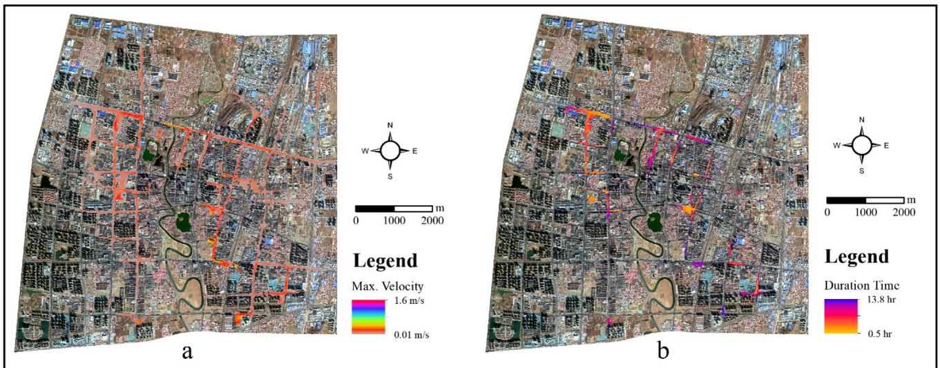
**Figure 8.** (a) Spatial distribution of the maximum velocity under a 3-year return period; (b) spatial distribution of the inundation depth above 40 cm under a 3-year return period.
