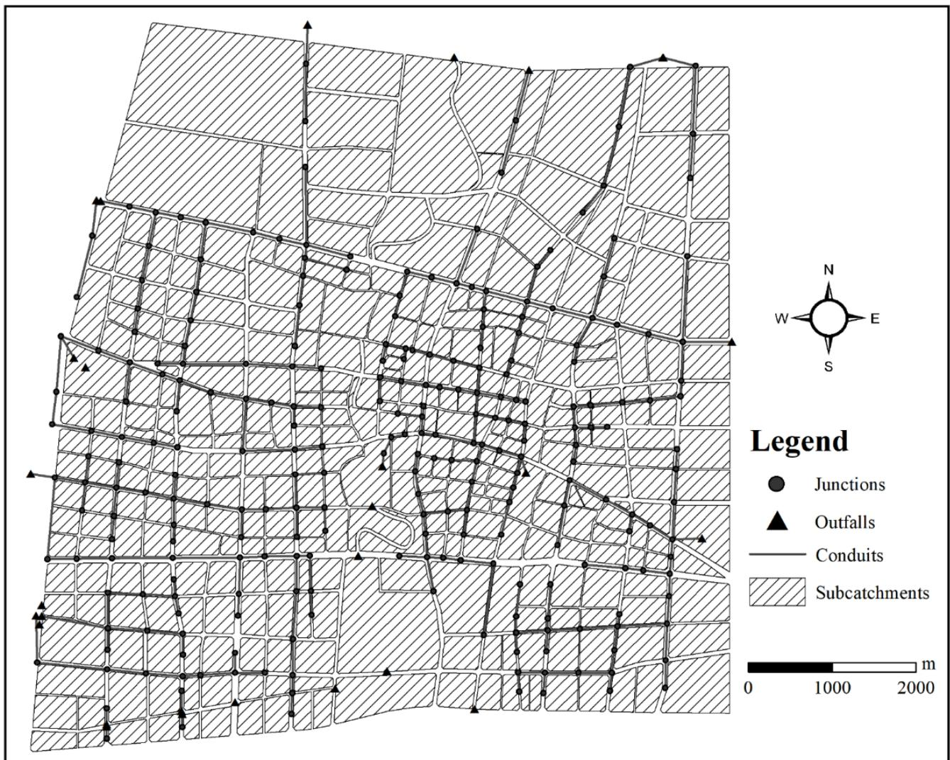
**Figure 4.** Generalization results of the SWMM model and the topological relationship of the pipeline.
