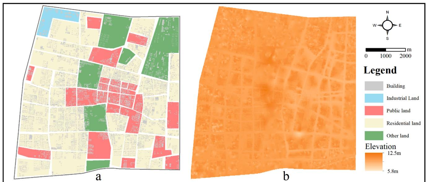
**Figure 3.** (a) Buildings extracted from GF-2 data and land-use type in the study area; (b) modified DEM based on buildings.
