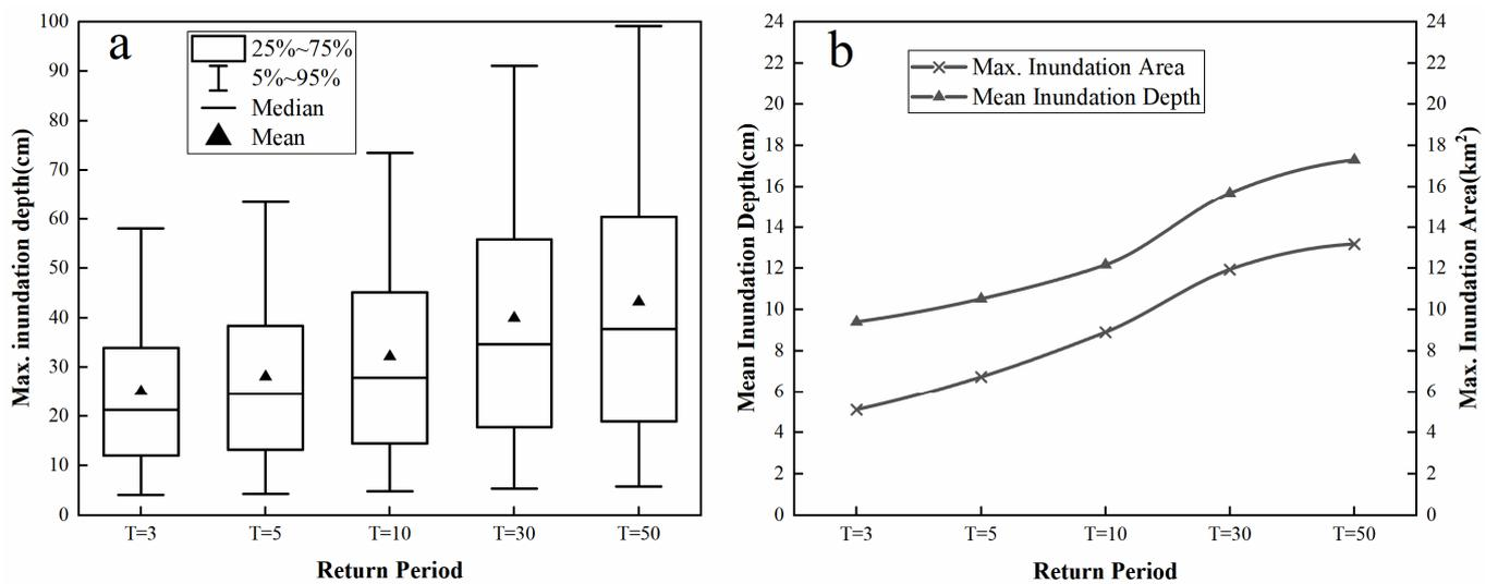
Figure 7. (a) Boxplots of the maximum inundation depth distribution under different return periods; (b) mean inundation depth and maximum inundation area under different return periods.
