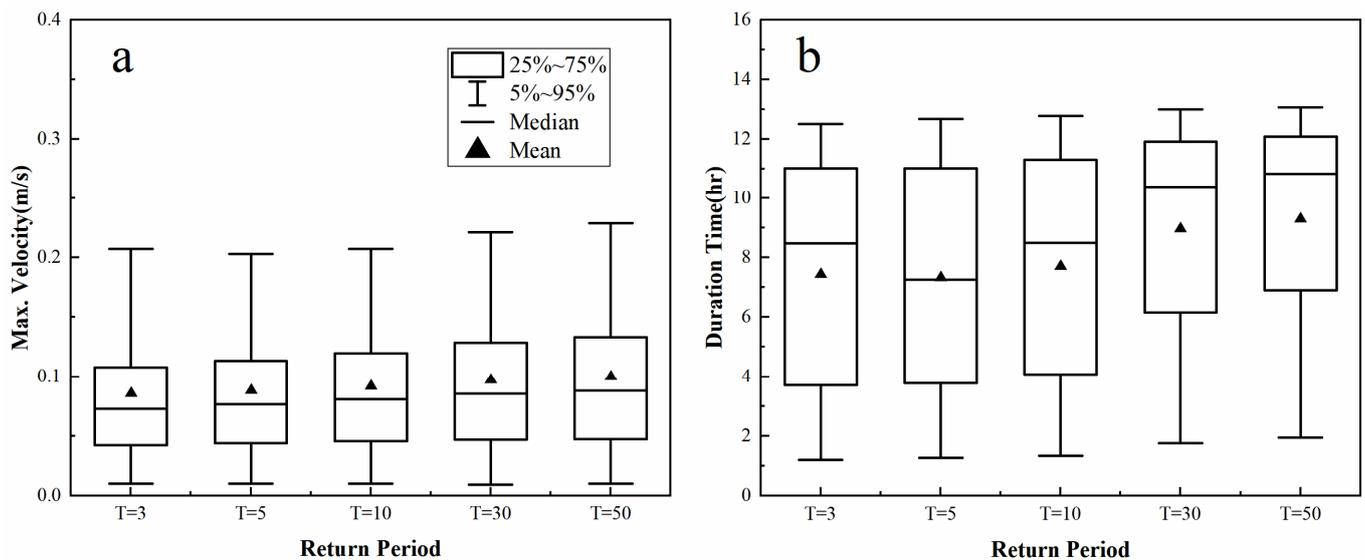
**Figure 9.** (a) Boxplots of the maximum velocities under different return periods; (b) boxplots of the duration time distribution of the inundation depths above 40 cm under different return periods.
