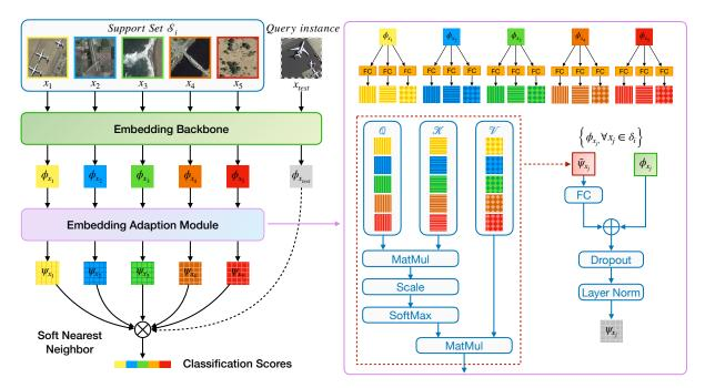
**Figure 5.** Illustration of the structure of our embedding adaption module, implemented with a set-to-set function based on Transformer. The right part shows the adaption step that transforms the embedding  $f_{\phi}(x)$  to  $f_{\psi}(x)$ . For notational simplicity, we use  $\phi_x$  and  $\psi_x$  instead of  $f_{\phi}(x)$  and  $f_{\psi}(x)$  in the figure, respectively.
