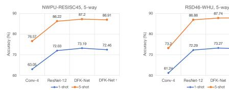
Figure 9. Few-shot classification accuracy of our model using different embedding networks on the NWPU-RESISC45 and RSD46-WHU datasets.
