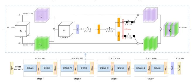
Figure 4. Schematic for the proposed Dynamic Kernel Fusion Network (DKF-Net).
