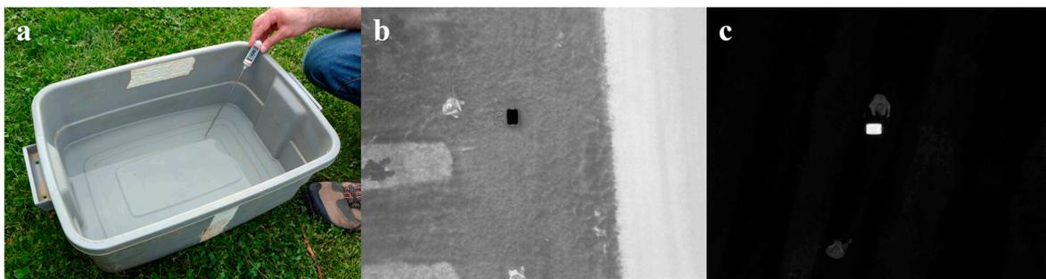
**Figure 3.** Illustration of the thermal camera calibration: (a) temperature measurement of the thermal camera calibration target with a digital thermometer; (b,c) example thermal images containing the calibration target before cropping taken at  $10^\circ\text{C}$  and  $75^\circ\text{C}$  water temperatures.
