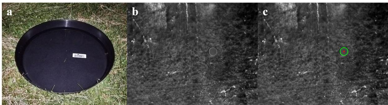
**Figure 5.** A ground control point (GCP) for georeferencing thermal mosaics: (a) in the orchard, (b) its appearance in a thermal image, and (c) being detected by our algorithm.
