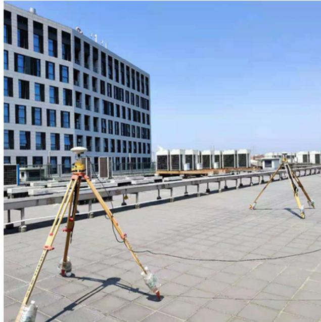
**Figure 1.** Photographs of the dual antennas on the roof of a building.
