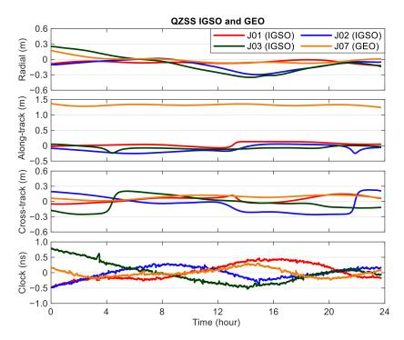
**Figure 8.** Epoch-wise orbit and clock differences for QZSS GEO and IGSO satellites between GFZ and WHU precise products on DOY 122 of 2020.
