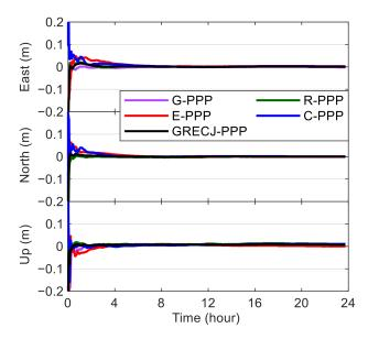
**Figure 10.** Epoch-wise position errors of static PPP using ESA final precise products at station KIR0 on 17 May 2020.
