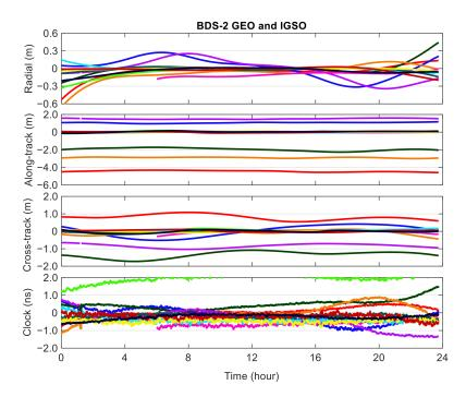
$\textbf{Figure 6.} \ Epoch-wise \ orbit \ and \ clock \ differences \ for \ BDS-2 \ GEO \ and \ IGSO \ satellites \ between \ GFZ \ and \ WHU \ precise \ products \ on \ DOY \ 122 \ of \ 2020.$
