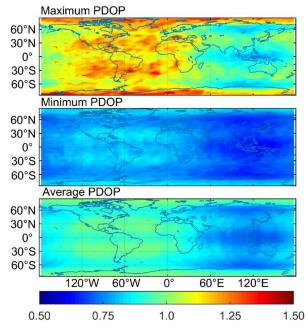
**Figure 2.** Global maps of maximum, minimum and average PDOP values for five-system combination on DOY 122 of 2020.
