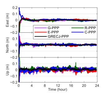
**Figure 12.** Epoch-wise position errors of kinematic PPP using ESA final precise products at station KIR0 on 17 May 2020.
