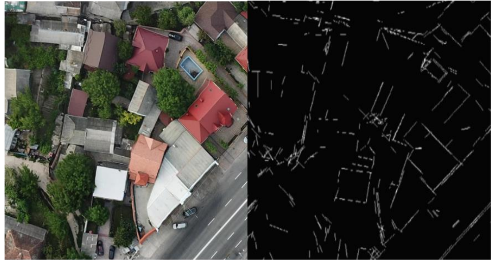
Figure 2. The visualized result of edge auxiliary information extraction. Left: the input (UAV) image. Right: the extracted information.
