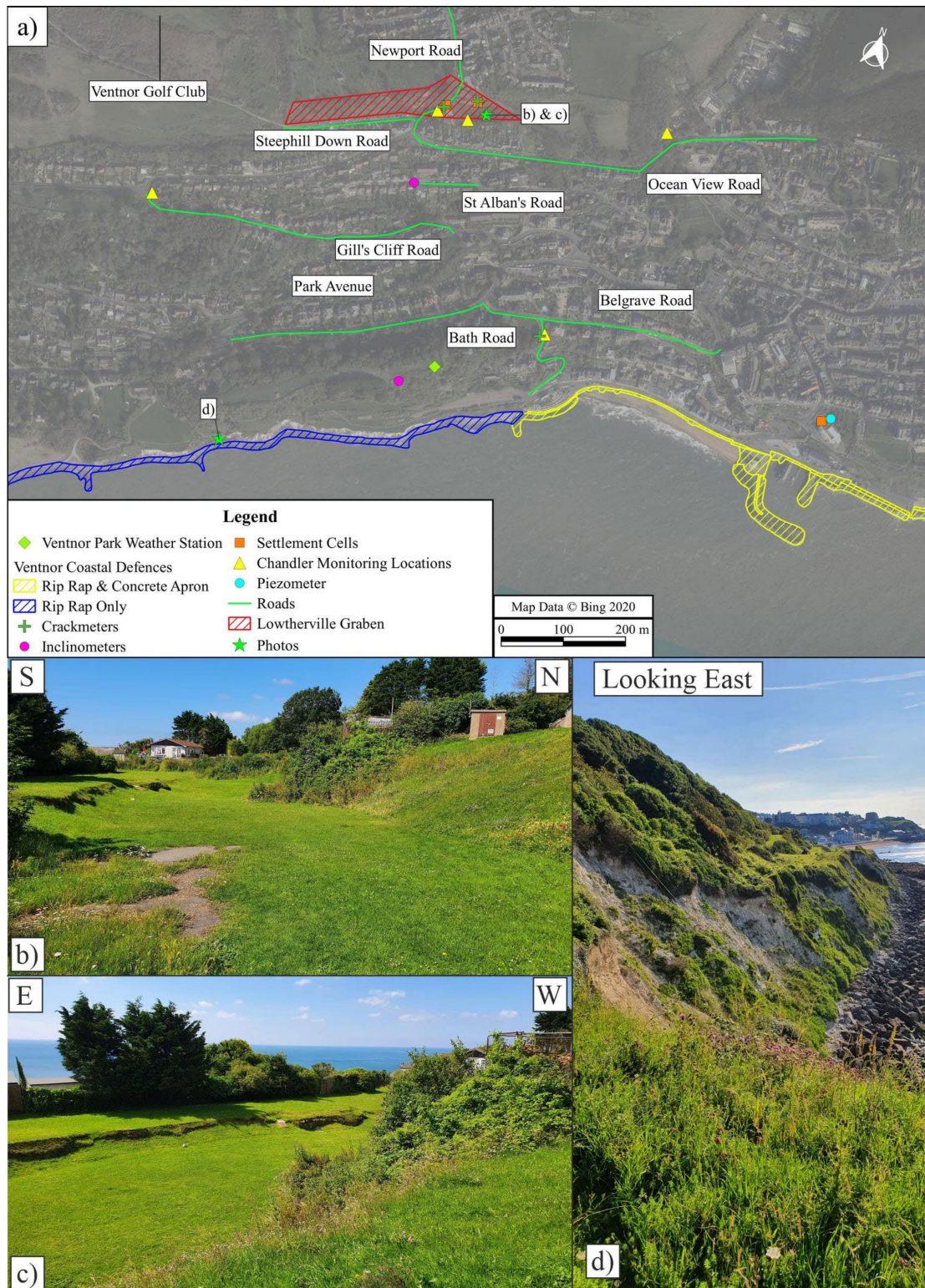
Figure 3. (a–d): Instrumentation locations at Ventnor, after Chandler [28], Geomorphological Services Limited [29], and Moore et al. [30] (a). Image shows the transition between rip rap and/or the concrete apron and rip rap only along the coastline. Image (b,c) shows ongoing movement at the Lowtherville Graben, showing settlement in the middle of the Graben that creates ca. 8 m tall berm to the north and 0.5 m to the south. Image (d) shows the toe of the landslide, with a rock apron present along the shoreline. The steep angle of the chalk cliff demonstrates the active erosion at the site. Image (a) created on QGIS with background imagery from Bing Maps (2020).
