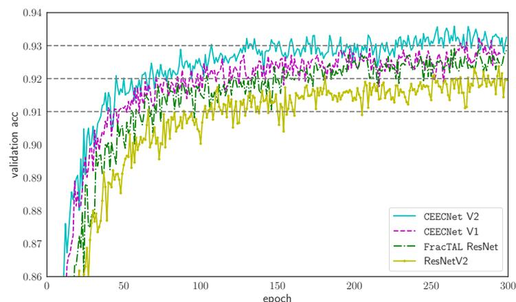
**Figure 9.** Comparison of the V1 and V2 versions of CEECNet building blocks with a FracTALResNet implementation and a standard ResNet V2 building blocks. The models were trained for 300 epochs on CIFAR10 with standard cross entropy loss.
