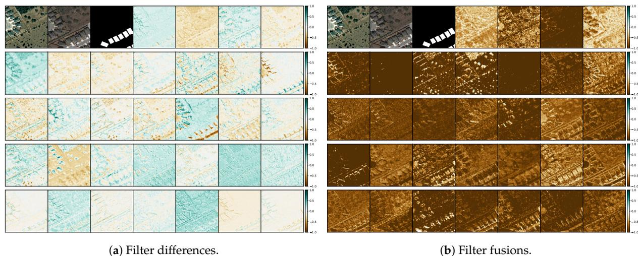
**Figure 20.** For the same model as in Figure 19, we plot the difference of the first feature extractor blocks (left panel) vs. the first Fusion feature extraction block (right panel). The entropy of the fusion features is half that of the difference channels. This means there is less “surprise” in the fusion filters in comparison with the difference of filters for the same trained network.
