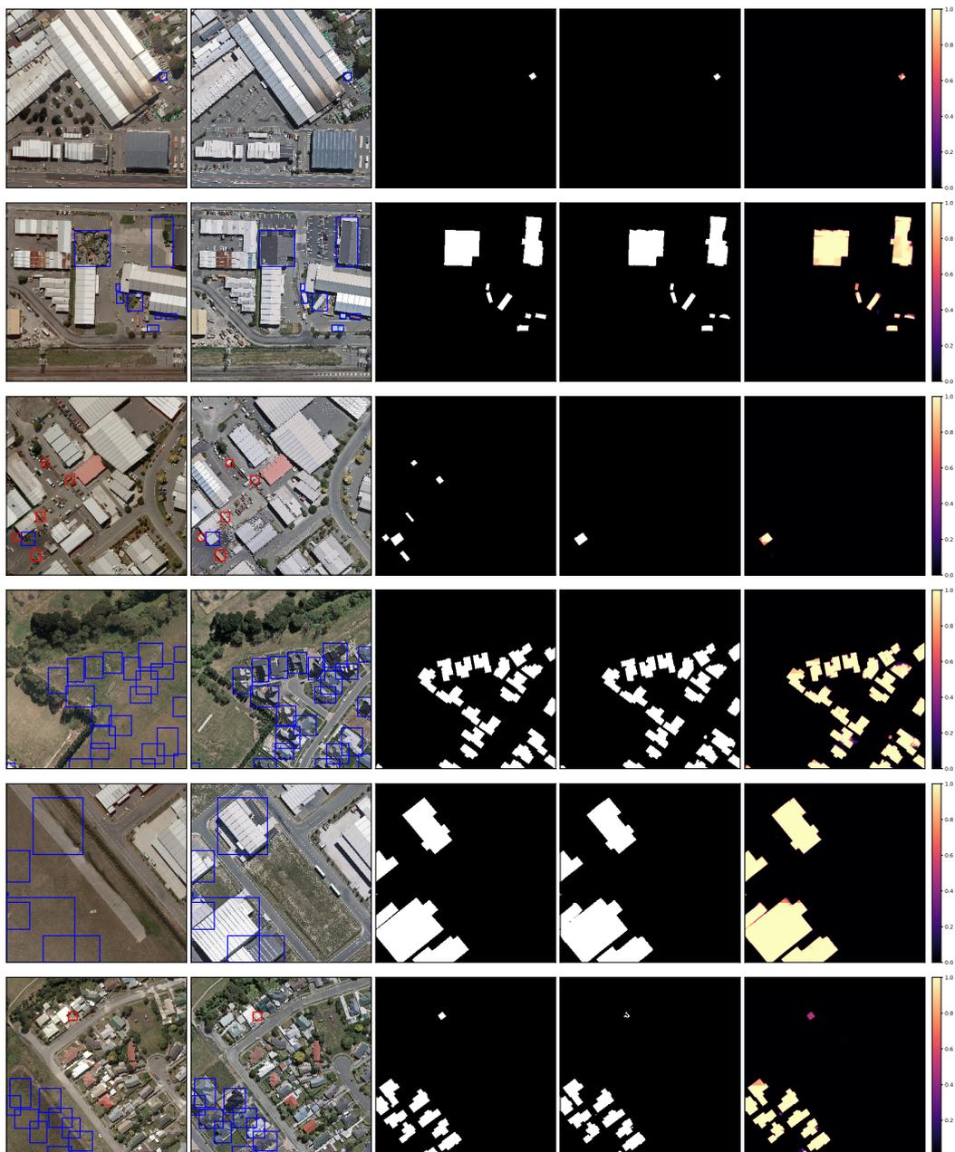
**Figure 14.** A sample of change detection on windows the size of  $1024 \times 1024$  from the WHU dataset. Inference is with the mantis CEECNetV1 model. The ordering of the inputs, for each row, is as in Figure 13. We indicate with blue boxes successful findings and with red boxes missed changes on buildings.
