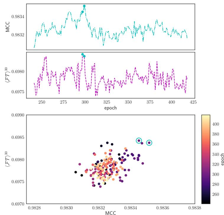
**Figure 8.** Pareto front selection after the last reduction in the learning rate. The bottom panel designates with open cyan circles the two points that are equivalent in terms of quality prediction when both MCC and  $\langle \mathcal{FT} \rangle$  are taken into account. The top two panels show the corresponding evolutions of these measures during training. There, the Pareto optimal points are designated with full circle dots (cyan).
