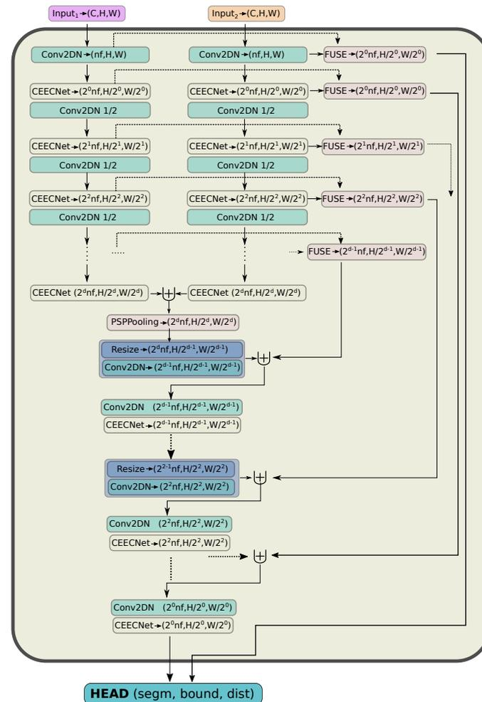
**Figure 5.** The mantis CEECNet V1 architecture for the task of change detection. The Fusion operation (FUSE) is described with MXNET/GLUON style pseudocode in detail on Listing A.3.
