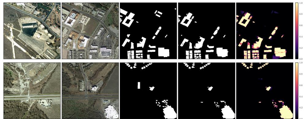
**Figure 13.** Examples of inferred change detection on some test tiles from the LEVIRCD dataset of the mantis CEECNetV1 model (evolving loss strategy, FracTALdepth  $d = 5$ ). For each row, from left to right, input image date 1, input image date 2, ground truth, change prediction (threshold 0.5), and confidence heat map.
