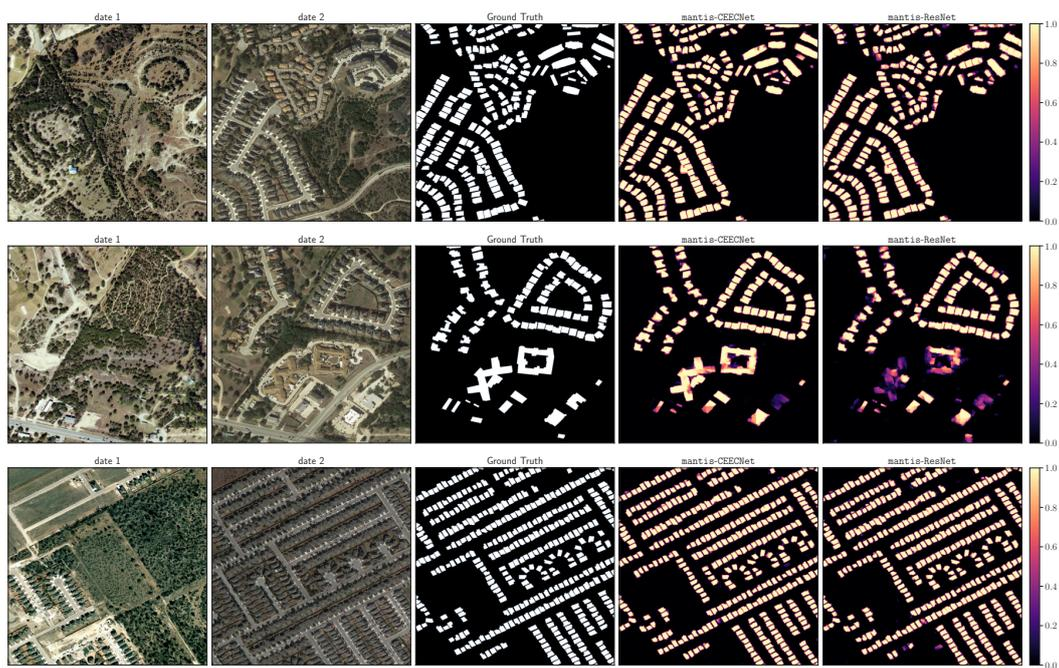
**Figure 17.** Samples of relative quality change detection on test tiles of size  $1024 \times 1024$  from the LEVIRCD dataset. For each row from left to right: input image date 1, input image date 2, ground truth, and confidence heat maps of mantis CEECNet V1 and mantis FracTALResNet, respectively.
