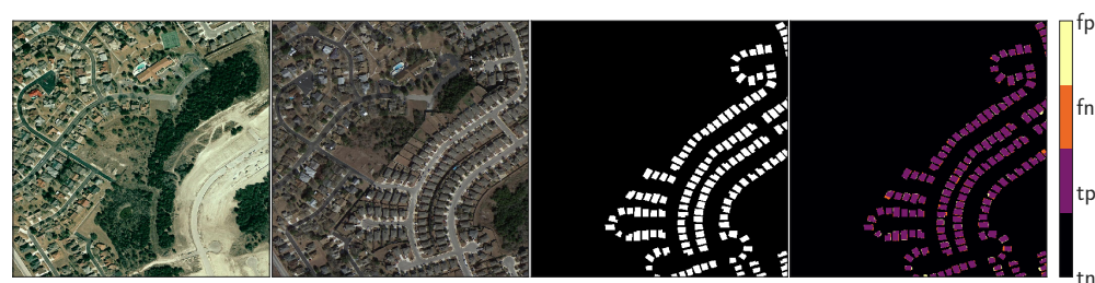
Figure 1. Example of the proposed framework change detection performance on the LEVIRCD test set [1] (architecture: mantis CEECNetV1). From left to right: input image at date 1, input image at date 2, ground truth buildings change mask, and colour-coded the true negative (tn), true positive (tp), false positive (fp), and false negative (fn) predictions.
