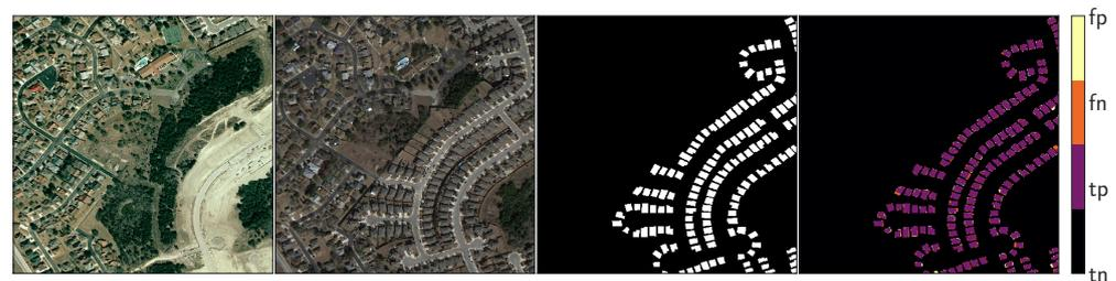
**Figure 1.** Example of the proposed framework change detection performance on the LEVIRCD test set [1] (architecture: mantis CEECNetV1). From left to right: input image at date 1, input image at date 2, ground truth buildings change mask, and colour-coded the true negative (tn), true positive (tp), false positive (fp), and false negative (fn) predictions.
