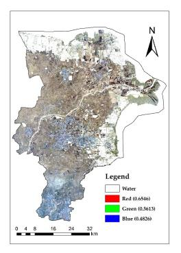
**Figure 4.** Dongying true color image after water masking with MNDWI. Within the boundary of Dongying vector, the white area is water, which has the same value as the background, and the non-water area is stretched according to the red, green, and blue band.
