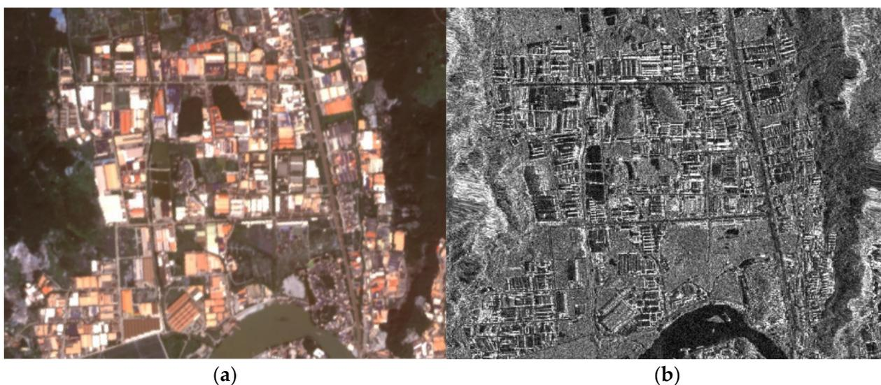
**Figure 1.** A typical optical satellite image (a) and its corresponding SAR image (b) of the same area.
