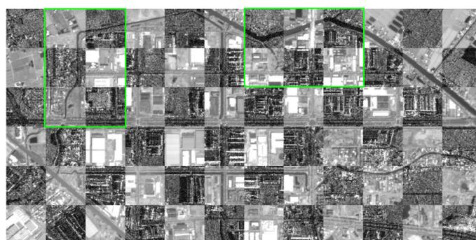
(b) The result of GF-1 image after geometric orientation.
