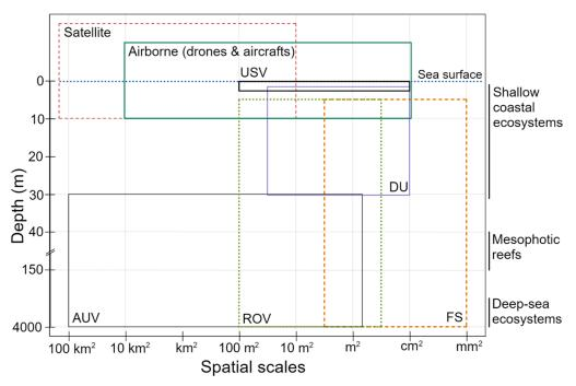
**Figure 1.** Present spatial scales of observation for hyperspectral imaging platforms in a marine context. This highlights the spatial extent to which each system can optimize its observations, plotted against the depth range of the system. Acronyms are defined by: unmanned surface vehicle (USV), diver units or systems (DU), autonomous underwater vehicle (AUV), remotely operated vehicle (ROV), and fixed stations (FS). Airborne includes drones and manned aircraft.
