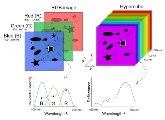
**Figure 3.** Comparison in the amount of information provided by an RGB image and a hyperspectral image cube from a heterogenous seafloor area.
