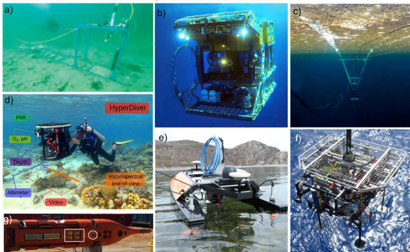
**Figure 4.** Photographs of platforms employed for in situ UHI studies. From (a–g), (a) electric rail, (b) remotely operated vehicle (ROV), (c) under-ice sled, (d) diver-operated unit (DU), (e) unmanned surface vehicle (USV), (f) fixed stationary platform (FS), and (g) autonomous underwater vehicle (AUV).
