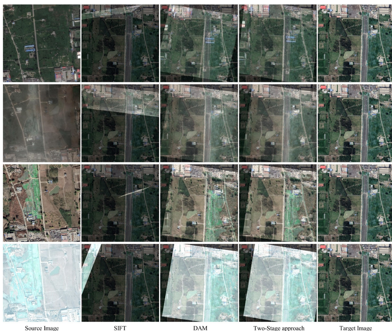
Figure 15. Registration of a group of multi-temporal remote sensing images from other times and region. Rows are each as follows: (1) the source images, (2–4) overlays of the target image and the result warped by SIFT, DAM, and ours, respectively, (5) the identical target images taken in 2020.
