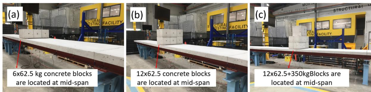
**Figure 8.** (a) first load 375 kg, (b) second load 750 kg and (c) third load 1100 kg.
