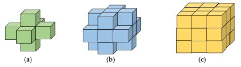
Figure 9. The adjacency criterion. (a) 6 adjacency; (b) 18 adjacency; (c) 26 adjacency.
