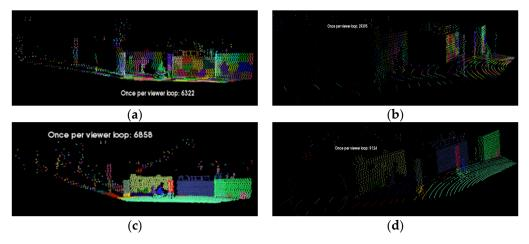
**Figure 18.** Region growth results of voxel clustering and hypervoxels' segmentation results. (a) Small-scale view; (b) Large-scale side view; (c) Small-scale view; (d) Large-scale side view.
