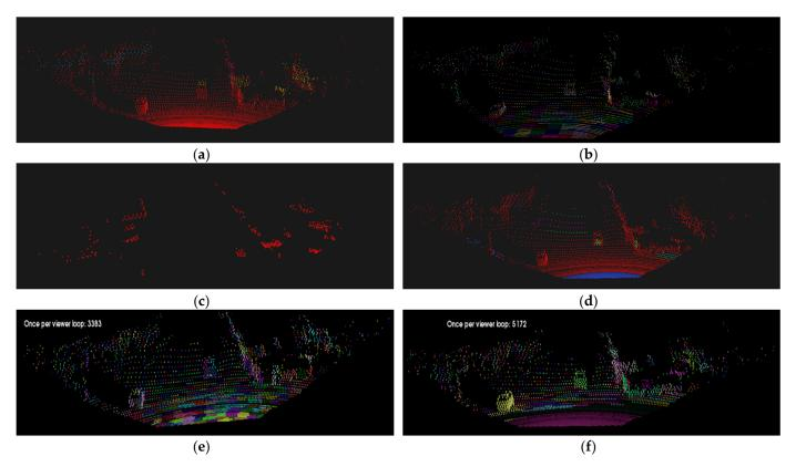
**Figure 19.** Segmentation results of different methods. (a) Color-based region growth method [38]; (b) Peer hypervoxel method [39]; (c) Minimum cut of graph model method [40]; (d) Distance grow method [41]; (e) Octree voxel method [42]; (f) Our result.
