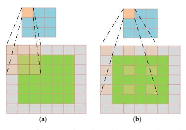
Figure 7. Different types of convolution. (a) Normal convolution; (b) dilated convolution.
