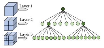
Figure 8. The octree structure.
