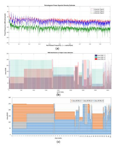
**Figure 20.** The spectrum and the RGB distribution of the object classes for segmentation detection results. (**a**) The spectrum of voxelized over-segmentation result; (**b**) The RGB distribution of the object point cloud class detection; (**c**) The RGB distribution of object class detection with functional semantic information.
