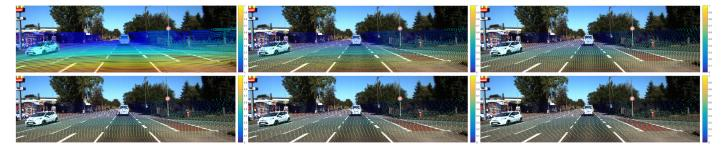
**Figure 13.** Multi-mode pre-fusion and alignment of 3D point clouds and 2D images under different sampling thresholds. The image shows the results for the threshold of the first few odd digits, i.e., the point cloud mapping map, in which the colorbar represents the depth of field, the warm color represents a close range, and the cold color represents a long range.
