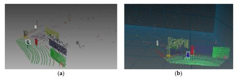
**Figure 22.** Mapping of the minimum object bounding box in point cloud segmentation of fusion data. (a) Mapping in side view for ROS rviz shown without grids; (b) Mapping in frontal view for ROS rviz shown in grids.
