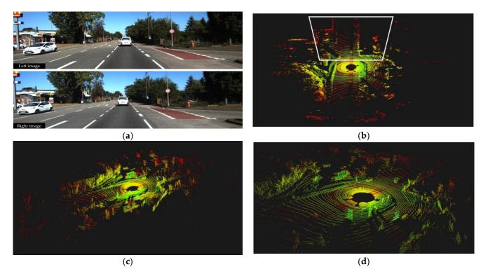
**Figure 12.** 2D and 3D data of the binocular color camera sensor and Lidar senor, respectively. (**a**) Stereo images; (**b**) top view of the point cloud (the trapezoid frame is the corresponding driving perspective area of the vehicle); (**c**) side view of the point cloud; (**d**) large-scale view of the point cloud.
