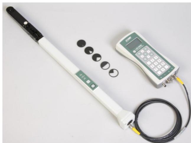
**Figure 3.** The LAI-2200C canopy analyzer.
