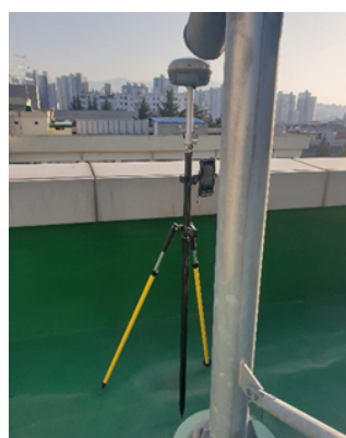
Figure 4. Image of field survey with Trimble R8s for measuring RTK measurement point.
