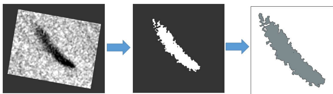
Figure 5. Left—is the preprocessed raw data: result after speckle filtering and geometric correction. Middle—is the masked oil spill area after processing and clustering the SAR image based on a predefined threshold of 2 decibel. Right—is the vector conversion of the raster oil spill mask to be enable area and other geographical calculations.
