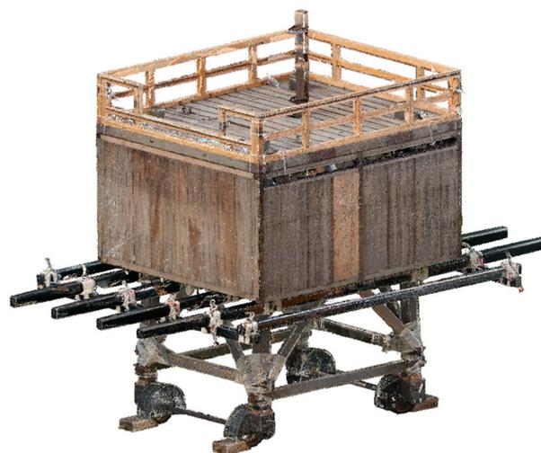
**Figure 16.** 3D-laser-scanned point cloud of the Hachiman-Yama float used in the Gion Festival in Kyoto City, Japan (7,866,197 points).
