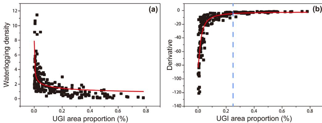
**Figure 7.** The logarithmic fitting (a) and the derivative (b) between UGI area proportion and waterlogging. The red line indicates the nonlinear fitting curve and the derivative curve, and the blue dashed line represents the threshold value.
