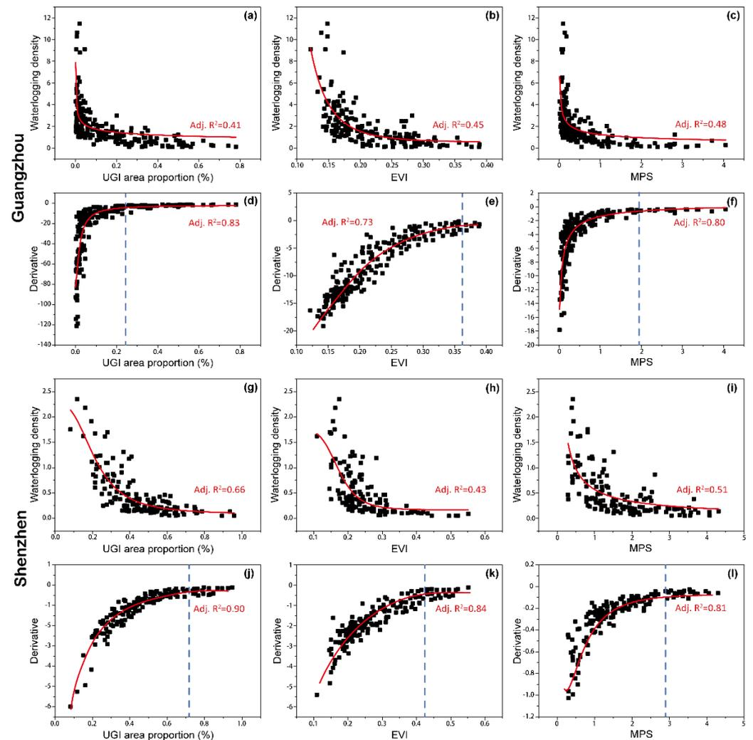
**Figure 11.** The relationship between UGI variables and waterlogging for (a–f) Guangzhou and (g–l) Shenzhen. The red line indicates the nonlinear fitting curve and the derivative curve, and the blue dashed line represents the threshold value.
