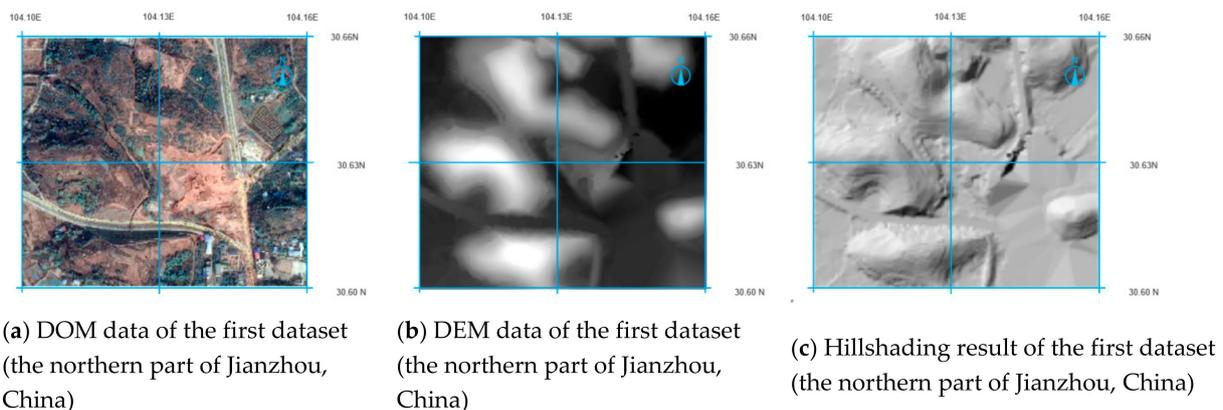
**Figure 8.** Experimental results for Dataset 1: (a) DOM data for Dataset 1 (Jianzhou); (b) DEM data for Dataset 1 (Jianzhou); (c) Hillshading results for Dataset 1 (Jianzhou).
