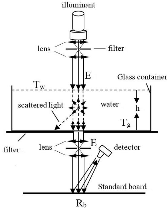
**Figure 6.** Schematic diagram of an optical parameter measuring device.
