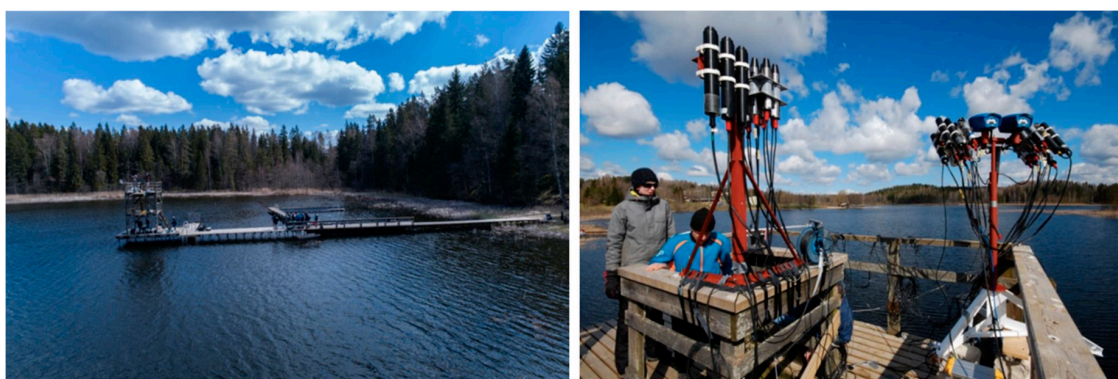
Figure 10. Pier and diving platform at the southern coast of Lake Kääriku with all the radiance (right) and irradiance radiometers (left) mounted in common frames for the outdoor experiment.
